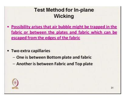
Possibility arises that air bubble might be trapped in the fabric or between the plate and the fabric which can be escaped from the edge of the fabric. Now, the problem is that here suppose this is the plate on which the fabric is being placed. And air bubble can be there between fabric and the plate, and also air bubble is present within the fabric also. So, during the transmission, it will affect the result.
