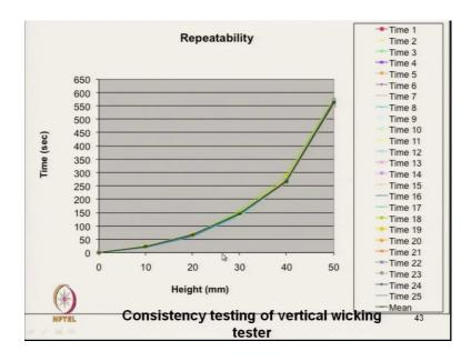
Now, here what we have tested the consistency of vertical wicking tester. And we have tested a particular fabric. And this fabric is tested 25 times, there are different time that fabric is tested. And what we have achieved we have achieved the exactly same reading. So, these curves are simply over lapping, which shows the repeatability of this tester say consistency of the testing of vertically wicking tester.
