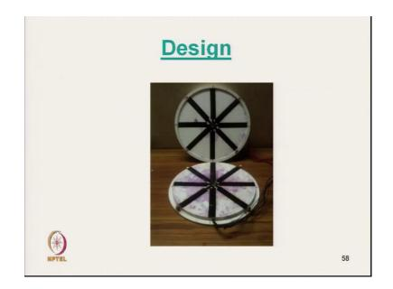
And this is the design of the instrument. So, this is here its inner side of the bottom plate inner side of the top plate. And the black tape is actually placed to prevent the parallel plate from wetting, because liquid will flow through this surface, and fabric is placed in between these plates.
