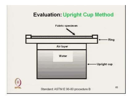
And the ASTM method which is the exactly same method exactly similar, which is called upright cup method. Similarly, upright cup is there earlier case it has a dish, it is air layer it is partially filled with water, and there will be fabric specimen.
