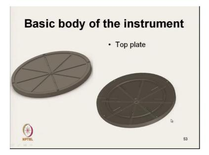
Now, this is the top plate, top plate inner side and this is outer side. Inner side we have slots.
