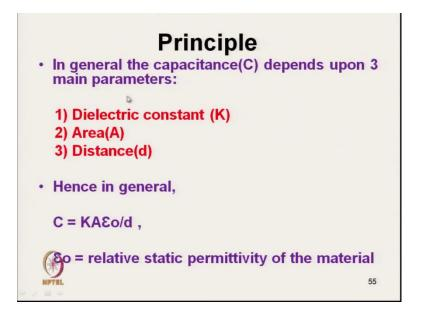
And in general the capacitance depends on 3 main parameters, one is dielectric constant K, second is area, and third is distance between. So, hence in general
