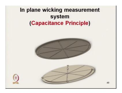
Next is that in plane wicking system using the capacitance principle. Till now what we have discussed it was resistance principle. Now, we will discuss one instrument which works in capacitance principle. These are the two plates insulating plates with slots. So, we have 1, 2, 3, 4 slots which makes actually 8 different directions, 1, 2, 3, 4, 5, 6, 7, 8 directions.
