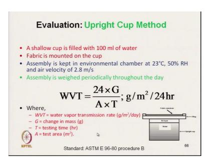
And in up right cup method, a shallow cup is filled with 100 ml of water. This is shallow cup it is filled with 100 ml of water. Fabric is mounted on the cup. Assembly is kept in environmental chamber at 23<sup>o</sup>C. Here temperature and relativity humidity is specified,
