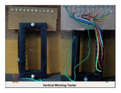
So, this is the actual setup. It is a holder fabric holder, and this is the circuit, and here these are the LED lamp.
