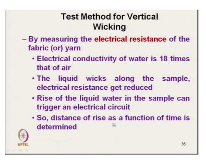
So, the alternate method is that by measuring the electrical resistance of fabric or yarn. So, we can measure the vertical wicking by measuring the electrical resistance. The electrical conductivity of water is approximately 18 to 20 % to that of air. So, typically it is 18 times to that of air which means if the air inside the yarn and fabric, if it is actually replaced by water during wicking, the conductivity of the material will increase.
