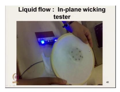
And here this picture demonstrate how the liquid is flowing, and the LED is glowing. So, we can develop the instrument commercial using this principle.
