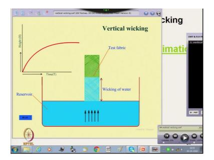
Now, if we see the animation here, this is reservoir here. And fabric is placed this is the test fabric. We are putting the fabric on the on the reservoir. And as soon as the bottom portion is in touch with the reservoir, water is wicked at certain height. And with the time we can plot the wicking height versus time. So, this we can plot manually. And there are other techniques where we can use the electronic method of measurement the wicking
