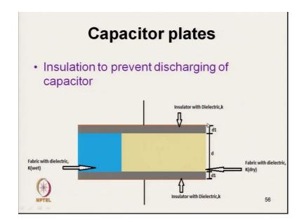
And insulation to prevent the discharge of the capacitance, we need to insulate. So, what you have done, we have used the material the plate which is insulating in nature, and the conducting plate, the metallic plate, is placed under slot. And here once it is flowing, the liquid is flowing, the liquid the water is actually replacing the air inside the fabric structure.
