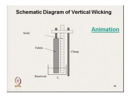
Now, this is the test system. This is fabric and reservoir is there and scale.
