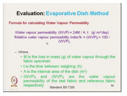
So, another method which is exactly same as that of earlier method that we will discuss, so evaporative dish method. The formula for calculating the water vapor permeability is
