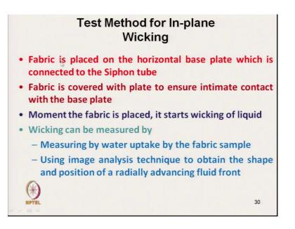
And the fabric is placed on the horizontal base plate which is connected to the Siphon tube as I have shown that is Siphon tube is there. Fabric is covered with plate to ensure intimate contact with the base plate. Moment the fabric is placed, it starts wicking of liquid. The wicking can be measured by measuring water uptake by the fabric sample, or using image analysis technique to obtain the shape and position of the radially advancing fluid front.
