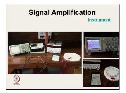
So, this is the instrument. And here this system, it is a top plate; and below that there will be bottom plate. And the electronic circuit, here it is actually recording the capacitance value change in capacitance value from 8 different parallel plate capacitors.
