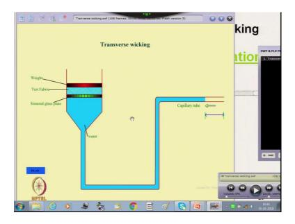
Here this blue colour which shows the water ok. And this is the capillary tube. And here this green colour - this plate, it is a sintered glass plate with pores. If we start, so after that this the fabric will be placed on the sintered plate. So, the fabric is placed onto the sintered glass plate and then we are plating we are placing another plate just to ensure the proper contact. After that placing, so the water will be wicked through the cross section of the
