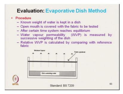
So, and in addition to that another method will discuss which is permetest. So, this method we will discuss one by one first is that evaporative dish method which is very commonly used. Here in this method there is a dish partially filled with water. So, known weight of water is kept in a dish. So, we can take that mass of the water, and open mouth of the dish is covered with the fabric specimen. So, this is the fabric specimen.
