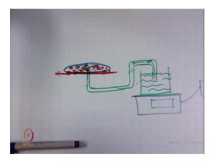
In this system, suppose this is the fabrics specimen at the center, we have certain hole. And the water is supplied through the centre of this. At the centre the water is supplied here, and this is actually it is a flexible tube, this is a system ok.
