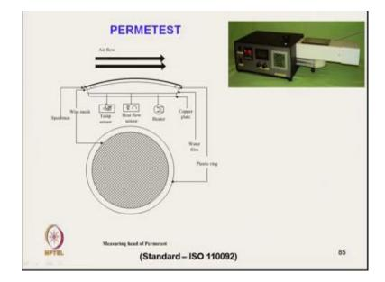
So, that is why the ratio is the relative water vapour permeability and this is the equipment. Here, we can see in this equipment. This one is the wire mesh. It is shown in the top view its wire mesh is there; on the wire mesh, we are placing the fabric. This is a fabric specimen, it is placed. Now at the bottom here it is a copper plate and then on the copper plate it is a water film is produced. So, water film is actually created on the copper plate and copper plate this plate is heated.
