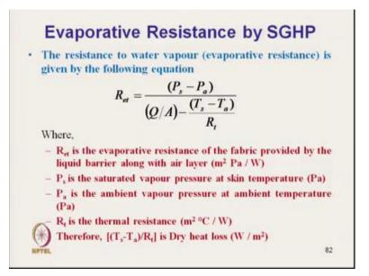
The resistance to water vapour that is evaporative resistance is given by the following equation.
