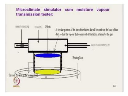
So, hear a circular portion of the fabric ok, it is placed here and this is the mimic skin; Humidity Sensor is here is placed.
