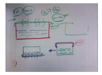
Now, if you see here this is the cup ok. In this cup is partially filled with water and first this cup mouth of the cup is covered with its PTFE membrane which is waterproof, but breathable. It allows the moisture vapour and then, the fabric specimen is placed. This arrangement is actually preventing the wetting of the fabric.
