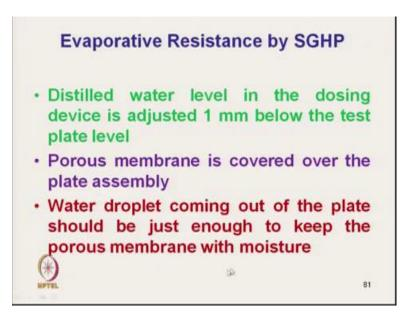
So, distilled water level in the dosing device is adjusted 1 millimeter below the test plate. So, otherwise the test plate will be flooded ok. The porous membrane is covered over the plate assembly. So, the test plate which is actually the sintered one; so, 1 millimeter below will keep the water level. And then, porous plate is covered with another porous membrane which will actually not allow the water to transmit through.
