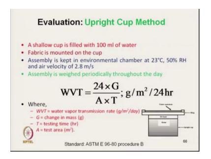
Assembly is weighed periodically throughout the day and we can calculate the water vapour transmission using this formula in terms of gram per square meter per 24 hour.
