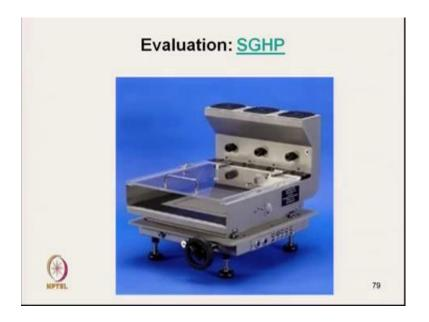
Next technique is that Sweating Guarded Hot Plate. So, we will discuss later when we will discuss the dry heat transmission, the guarded hot plate the principle of guarded hot plate we will discuss later. But at this point, we will see the principle of sweating guarded plate. The working principle is similar to that guarded hot plate, but with little difference where we use the sweating plate.
