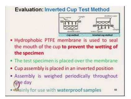
So, to do that the technique is that the hydrophobic PTFE membrane is used to seal the mouth of the cup to prevent the wetting of the specimen. So, once the fabric along with the cup is inverted. So, to prevent that wetting of the fabric specimen, the mouth of the cup is first covered with the PTFE membrane which is waterproof; but breathable. But then, the test specimen is placed over the membrane.
