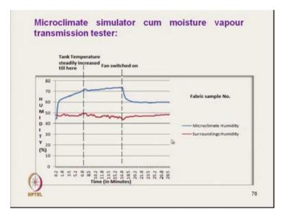
Now, this graph shows Microclimate humidity and surrounding humidity; if we see and this surrounding humidity and microclimate humidity is plotted with the time. We can see here the surrounding humidity is almost constant; it is not changing, but the microclimate humidity, it increases gradually with the time. That means, as the moisture vapour is transmitted through the mimic skin, the fabric has got its some the moisture
