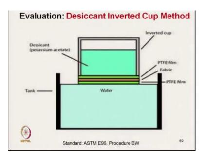
Now, after that another method is that it is called Desiccant Inverted Cup Method. Now this is almost similar to that of inverted cup method, but it has got some difference also. In inverted cup method, the cup was filled with water. But here we are not using any water; in place of water here we are using desiccant material.
