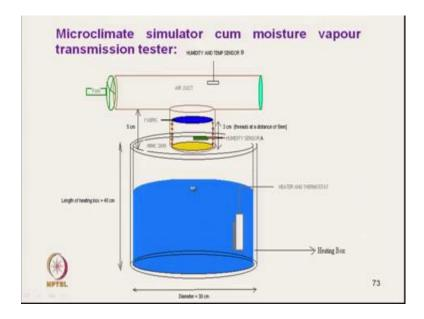
So, it simulate the micro climate and then it can measure the moisture vapour transmission. Now this is the instruments setup schematic diagram of the instruments. What is Microclimate? As we know the Microclimate is the climate between our skin and the fabric. So, we would like to know what is the micro climate condition for different fabric or different environmental condition and also we can calculate the moisture vapour transmission.
