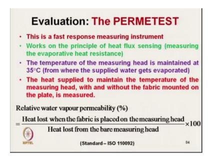
And this follow the standard ISO standard 110092 and this method its very fast response method. So, this is the fast response measuring instrument. It works on the principle of heat flux sensing that is measuring the evaporative heat resistance. The temperature of the measuring head is maintained at 35 degree Celsius. Again here we measure the measuring head temperature, 35 degree Celsius which is equal to our skin temperature from where the supplied water gets evaporated.
