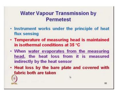
The instruments works under principle of heat flux sensing it sense the heat flux. Temperature of the measuring head is maintained in isothermal condition at 35 degree Celsius. When water evaporates from the measuring head, the heat loss from it is measured indirectly by heat sensor. Heat loss by bare plate and covered with fabric both are taken. (Refer Slide Time: 53:26)
