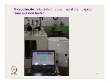
This is the actual photograph of the instrument and we can record the change of relative humidity and temperature with time.
