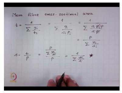
Mean fibre cross-sectional area. Now we have just now obtained t=gi/ti. If you remember from this module 1, fineness is related to cross-sectional area and density of fibre. How is the relation? The relation is fineness=cross-sectional area\*density. So we can write this, this we can write in terms of volume fraction, \*rho i/rho. So this rho is going there and then this gets cancelled. So what we obtain volume fraction/cross sectional area of ith component.
