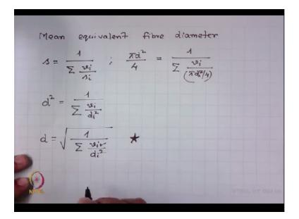
We have just now derived that the mean cross-sectional area of fibres in the blend is 1/volume fraction by the individual cross-sectional area. What is this s? s we can write as pi d square/4, where d is the mean equivalent fibre diameter in the blend which is equal to 1/volume fraction and si, pi di square/4. So we can write down that d square=1/summation volume fraction/di square.
