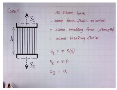
So, this is a case 1, very simple case, we assume all fibres have same force strain relation, all fibres have same force that is strain, they have same breaking strain. What does that mean? That means all fibres are identical so far their tensile characteristics are concerned, in such a situation the following relations are valid, we will be able to multiply them similarly, strength will be equal to strength of the bundle will be = number of fibres, n \* strength of one fibre.
