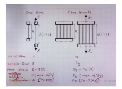
Here is one fibre and there is a fibre bundle, so what you see here, these are the jaws of a tensile tester, a fibre is gripped by both jaws of the tester and here the distance between the jaws is h, when you apply a force, capital S as a result, it elongates, so the length becomes h \* 1 + epsilon, where epsilon is the elongation similarly, we consider a bundle, an ideal fibre bundle where the initial distance between the jaws is h.
