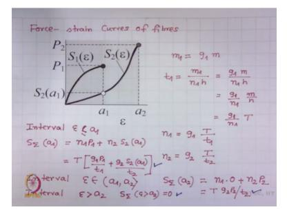
And there will be some subscript, there will be some variables without subscript, they are common to both now, we consider this kind of stress strain force strain curve of fibre, as I said you 2 types of fibres, one and two, suppose this is the force strain curve of type 1 fibre and this is the force strain curve of type 2 fibre, so type 1 and this will be type 2, this twisting behaviours of these fibres are very different.
