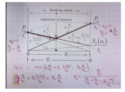
So, this is the graphical representation of this expression, this, let me explain you what is what in this diagram, x axis mass fractions are plotted, g1 denotes mass fraction of type 1 fibre, g2 denote mass fraction of type 2 fibre, when g1 = 1 at this point, mass fraction of type 2 fibre is 0, similarly at the end when g2 = 1, mass fraction of type 1 fibre is 0, it has 2 y axis, this y axis, we plot this point is basically P1/t1.
