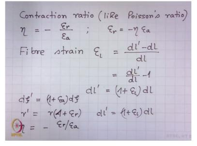
So we define contraction ratio is like Poisson's ratio, we use the symbol eta for that is = - radial strain / axial strain, this gives you – eta times this. The last quantity is fiber strain because of the application of force the fiber is also stressed, it also exhibits strain, so what is fiber strain? Fiber strain let us use this symbol epsilon L again it is defined by the ratio of change in fiber length / original fiber length.
