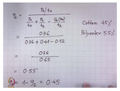
So the bundle tenacity will be minimum when g2 = P1/t1 / P1/t1 + P2/t2 - S2 a1/t2. So these data are given here. What is P1/t1? Is given as 0.36/0.36 + P2/t2 is given as 0.41 - S2 a1/t2 is given as 0.12. So this value will come as the ratio of 0.36 to 0.65 which is = 0.55 that means when, so g1 is 1-g2 0.45. When cotton fiber mass percentage is 45 and polyester mass percentage is 55, the resulting bundle gives the minimum strength.
