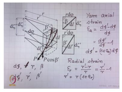
This diagram is very much related to the diagram that we discussed in the module of radial migration of fibers in yarn. What we see here is there is a general fiber element dl is its length, this element. So as we know from the module of radial fiber migration in yarn where we talked about general fiber path, fiber element, different angles. So this fiber element initial fiber element of length dl is characterized by 3 quantities.
