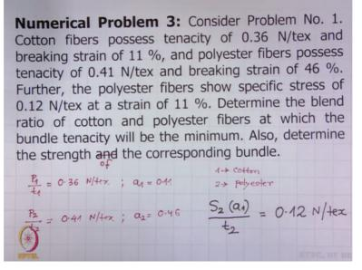
So this problem is basically an extension of problem number 1 of this module. You remember in problem number 1, this information was given, cotton fibers possess a tenacity of 0.36 Newton per tex, breaking strain 11%, polyester fibers possess tenacity of 0.41 Newton per tex and breaking strain 46%. Further the polyester fiber source specific stress of 0.12 Newton per tex at a strain of 11%.
