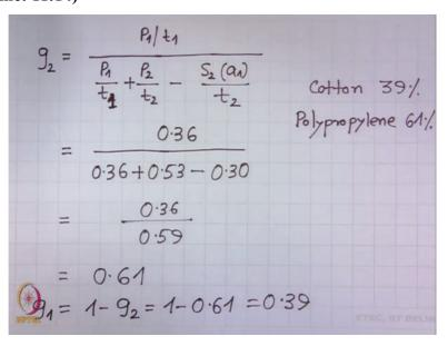
So the blend ratio at which bundle tenacity will be minimum is (()) (11:22) P1/t1 + P2/t2 – St a1/t1 is this. Now in this particular problem P1/t1 is given as 0.36, P2/t2 is given as 0.53 - S2 a1/t2 is given as 0.30 right. So what will be this value 0.36 / 0.59, so this will be = 0.61. Then what is g1? g1 is 1- g2. So 1 - 0.61. So 0.39, what does that mean? The blend ratio cotton 39%, polypropylene 61%.
