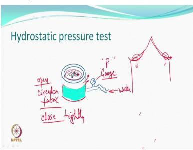
Like, you have this tented structure. And so, water can come and settle here. And may have a tendency to drip down. Right. So, under some amount of hydrostatic pressure, we would like to see how much water penetrates. Or we increase the pressure by any motorized system; and then see what happens. So, one of this test is that, these are 2 pieces. One at the bottom can be filled with water.
