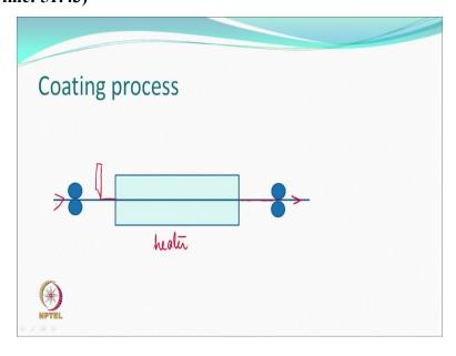
That you have a material. For example, here, you have applied something through a knife-on-air. For example, some very light material is coated. Then you pass through a heater. It can dry or cross link. And then, finally, what you have is very fine coating coming out on the textile. Alright. So, padding, we use only if you want both sides a complete immersion of the material. You can do both sides coating also; no issues.
