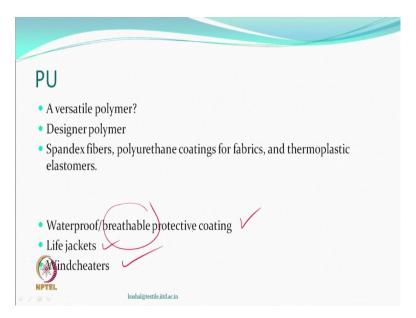
So, we can make waterproof, breathable, mentioned we will talk about later; life jackets, wind cheaters. Very thin coatings can do the job. And very lightweight. And that becomes an important. So, polyurethane is one of the interesting materials for using on textiles. So, in a nutshell, what have we talked about is;
