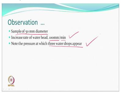
Let us say you have the sample size 50 mm diameter fabric. Increase the rate of water head, let us say at 100 millimeter of water per minute. And then, when 3 water drops appear, you stop the test and say: well, this is the pressure. And that becomes your hydrostatic pressure test. Right.
