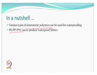
That various types of elastomeric materials including polyurethane can be used for making textiles waterproof. Right. Of course, other materials like PVC, we talked about. Similarly, PE, PP can be coated or applied in different ways; not necessarily it has to be coated only, you can apply different ways. So, that can make waterproof. As long as there is a layer which is called a film and there is a layer which is called a textile; so, it is a coated textiles.
