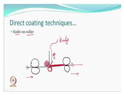
So, what it means that, if you want to control the thickness of the coating, then this type of technique can be used. Where by adjusting the distance between the roller and a knife which controls like a doctor blade. It controls and we call it a knife, which allows only a certain amount of solution or a foam or a latex to pass through. One simple diagram we can try and explain.
