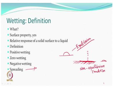
Spreading. Spreading is a situation. When you put a drop of water on a surface, within no time, it just gets absorbed. It is a very hydrophilic surface; and you put a drop of water. You just do not see. You are not able to measure the contact angle at all. You cannot measure the contact angle. You put a drop of water. And you see, immediately it spreads. So, cannot measure. So, this is in a way a non-equilibrium condition.
