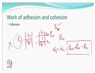
So, there are 2 more terms that we can talk about: work of adhesion and work of cohesion. Now, work of adhesion and cohesion mean that is a solid surface and liquid surface, liquid adheres to the solid. If it adheres to the solid more, then it will be, more work will be required to separate them, because they like each other. If they do not like each other, less work will be required to separate them. Right.
