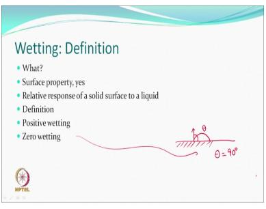
Zero wetting, like we just said before. What is a zero wetting? So, if it is a zero wetting; this is a surface and you put a drop. And if the contact angle is equal to 90 degrees; and if the contact angle is 90 degrees, then we consider a zero wetting. Okay.
