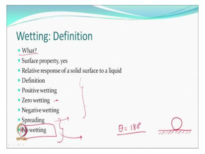
Yeah. No wetting. Remember, we should not confuse no wetting with zero wetting. Zero wetting is what? What? When theta is equal to 90 degrees. Zero wetting is on the other hand, where we expect the contact angle to be equal to 180 degrees. That just a spherical layer with a point contact. Its condition is very difficult to obtain in practical life. For various repellency requirements, we may be very happy with 120, 130, 140 degrees; very, very happy about that.
