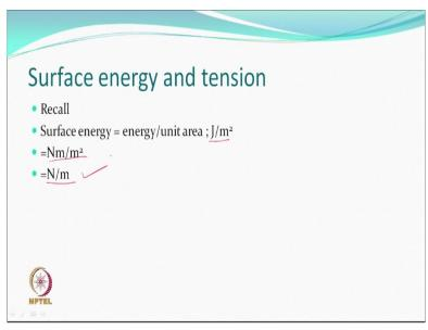
And then, this is, in a way can be expressed as newton meter per meter square, which is obviously, can be expressed as newton meter, newton per meter.
