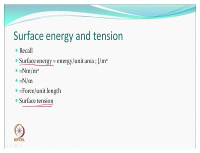
So, sometime, when somebody says, well, I am talking about surface energy modifications; or sometime they refer it to surface tension. So, they can be terms which are equivalent. But this surface energy is per unit area. And surface tension is per unit length, okay, the force per unit length. That is, energy per unit area, which becomes force per unit length. Now, this will happen.
