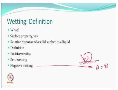
And then, we talk about negative wetting. So, negative wetting is when the contact angle is more than 90 degrees. This contact angle is an obtuse angle, then it is, then it is called negative wetting. Right. So, is there a significance of zero wetting? Well, actually, not really
