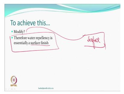
So, one important thing which we must remember that water repellency is going to be essentially a surface finish. So, what are we going to modify? Surface; we are going to modify surface. So, that is one difference, which you must remember. And therefore, we would be happy that the surface changes, but we are not blocking the pores or of the fabric or the interstices between the yarns.
