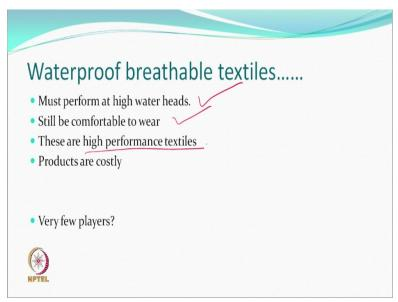
So, waterproof breathable textile, what do we expect? Must perform at high water heads. That is the pressure, at high pressures. And still, it should be comfortable to wear. And if you can do this; and which we will see how it can be done. Then they will be in the category of high performance textiles. So, they are special fabrics which will be used by at special conditions.
