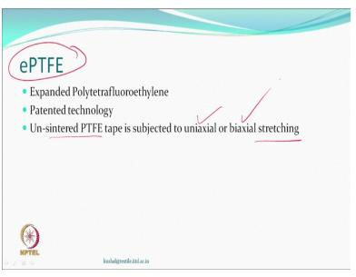
Is called ePTFE, which is called the, which is the expanded PTFE. It is a patented technology as far as the waterproof breathables are concerned. Interestingly, an un-sintered PTFE tape is taken and is subjected to stretching, either uniaxial or biaxial stretching.
