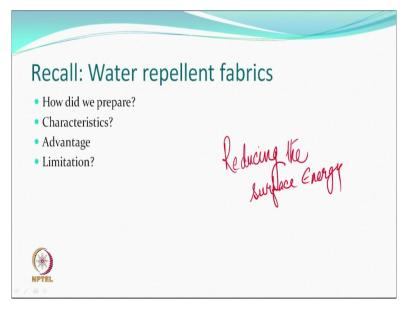
When we produced water repellent fabrics, what did we do? We made the surfaces, the surface of the fabric, a low energy surface. That became a water repellent. So, main characteristics are: That if you put a water drop, it will roll off. That is repellency. But it does not offer you any significant resistance to penetration of water. So, if it is a light rain, very, very light drizzle, it is fine.
