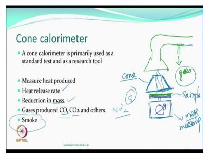
So these cone calorimeter actually burn the sample completely, they believe in that, so they are called cone because there is a cone where there are heating elements and certain amount of heat flux is generated a certain temperature is generated which could be 400 degrees 500 or whatever and theoretically there is a platform or a sample holder which is on some type of weighing machine, it is burnt because the heat flux is coming after the burn happens.
