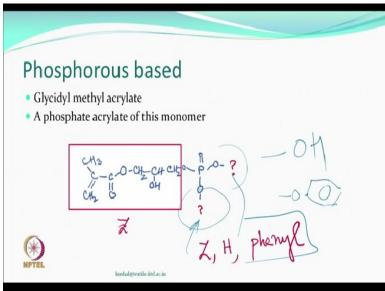
So another compound which is also based on a different group, but this is a reactive group and this reactive group again is an n methyl group and you have phosphorus here and other of course are the compound which have been attached or the groups which have been attached to the phosphonate to make it compounding. This became a very popular commercial compound as well called the Pyrovatex CP, that this was CP so there may be based on what you add to different parts of the hydroxyl group.
