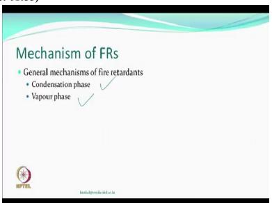
We also learnt general mechanisms which we called as condensation phase mechanisms or vapor phase mechanisms. So condensation phase means that the flame retardants will during the burning process alter the process of burning you know path of decomposition and the vapor phase is where all the gases are now there in the vapor phase free radicals are being formed and so you have to worry about either the free radicals or the heat release has to be taken away.
