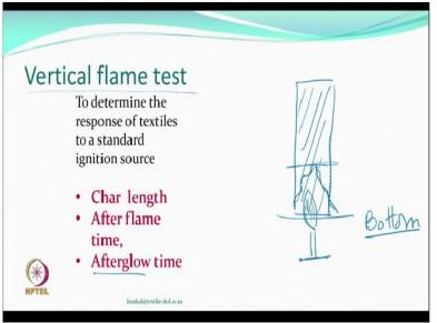
One is the vertical flame test you saw a small little video before which where the test was being done, a vertical flame test is one of the very severe tests a fabric can be subjected to burn from the bottom, what it therefore means is, if you burn from the bottom it is the serial it will go up and up and up, so if you burn the fiber for a certain period of time fabric for a certain period of time remove the flame you remember definition remove the flame and then measure.
