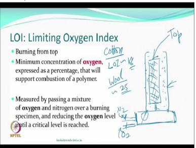
Another is a little more quantitative test more reliable called the limiting oxygen index test, so in this case you have created system where you can change the environment let us say the sample has been mounted inside a jar, this jar, this is the sample and you pass 2 gases oxygen and nitrogen, you know nitrogen does not burn oxygen helps to burn right. So mixture in the normal environment we have approximately about 21% oxygen, rest is nitrogen and other gases alright.
