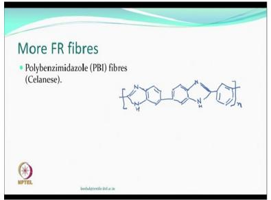
Not a very popular fiber but the PBI fibers are also very very highly heat resistant fibers you can see the leather structure, double bonded structure quite a lot and so by structure itself they are pretty stable and therefore inherently fire retardant.
