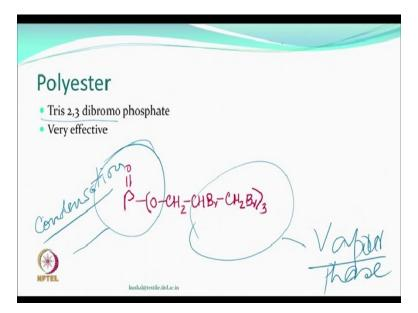
Another very interesting compound which is phosphorous compound, why we gain one and go to the phosphorus, the phosphorous and bromine combination also can be an interesting compound so part of it will work by the condensation phase mechanism, the other part would work with the vapor phase. So you have a dual action right. So if this compound is either as a finish is available on the fabric. So you remember there this is 3, so Tris 2 3 dibromo phosphate ok.
