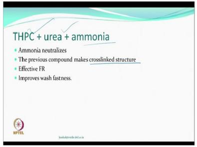
If you use THPC, urea and also ammonia which we neutralized so that chloride part will be taken care of reactions can take place, they can make cross-linked structures and therefore the wash fastness can be improved and this combination particularly for the cellulosic material have been found to be very very effective of flame retardant. Obviously we can appreciate this works generally by the condensation phase mechanism.
