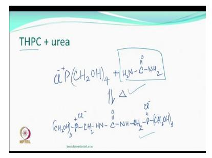
So one of the compound which we talked about last time was THPC tetrakis hydroxy methyl phosphonium chloride right. So in the presence of heat and in the presence of urea some such compounds are formed. So it's a large molecular compound and one can neutralize this also with another alkaline compound may be you could use ammonia itself, if you use ammonia then you can get cross-linked products.
