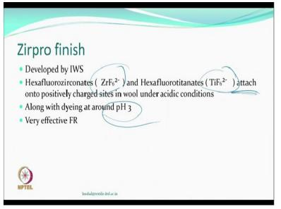
And called as zirpro finish, it is expected that in the acidic condition wool would have positive charge and this compound the fluoro compound with a zirconium and titanium are negatively charged. So they do get attached to the wool pH maybe if around this pH or maybe it is around that you can theoretically do exhaust dying as well as exhaust this finishing agent along with the dying.
