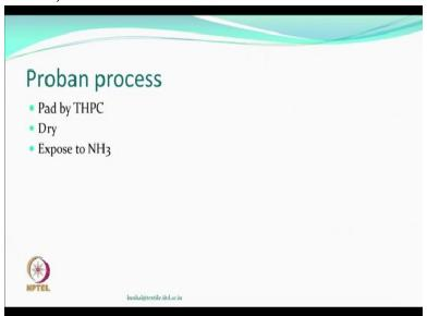
Another process which was commercialized and was known as a Proban process also used THPC ok, this Proban process also used THPC, so what you had to do was padded by THPC a solution dry and then during this process you expose it to the ammonia vapors and then the reaction would be there and in some sense there will be polymerization and cross-linking between the molecules and therefore the size will be more and it works.
