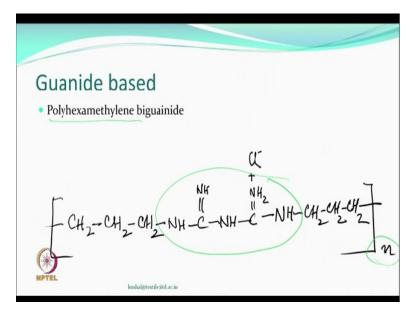
Now that guanide based compounds also have been suggested for antimicrobial activity for example a compound called the polyhexamethylene biguainide because of this here this is the biguainide structure and rest of course based on this plus charge, you would have either chlorine or bromine iron will be there. So it can be polymeric so even if it does not react it will still have a large molecular weight and so fastness cetera could be better.
