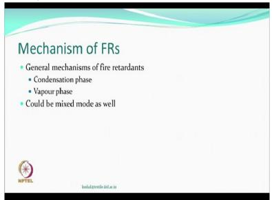
That is condensation phase mechanism which meant the flame retardant would participate in altering the path of decomposition or in the other case all the activity that happens for retardants happens in the flame, in the gas phase, so that called the vapor phase mechanism, some agents can work in both ways, in both by both mechanisms. So they could be called the mixed mode or a dual mode type of FRs as well.
