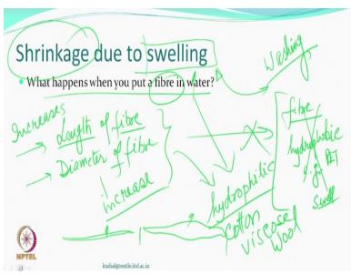
Another mechanism of shrinkage in any fabric including wool is due to swelling. Now, we again remember what are we talking about, we are talking about shrinkage during washing or laundering, not every type of shrinkage okay, which would mean swelling. If you put
