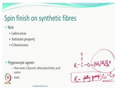
Spin finishes 3 roles lubrication, so that fiber, fiber friction, fiber to metal friction, fiber to ceramic guide friction all that is reduced because these yarns have to pass through different parts of the machines. Other important thing of course is antistatic properties, because synthetic materials can develop static charge as we understood and therefore, processing can be very
