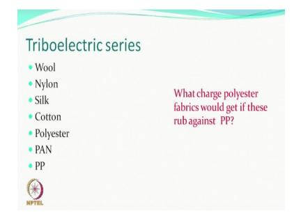
So, there is something called a triboelectric series, various types of generally non conducting electrically non conducting materials. They behave like dielectrics and they develop charge either positive or negative based on their surface, based on the ease with which the electron could be transferred, let us say when you rub 2 surfaces, one of the polymer fiber textiles may be able to you know give out more electrons.
