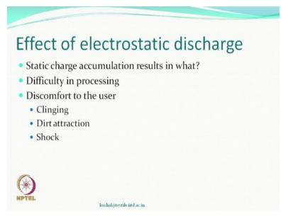
If charge accumulates obviously, whenever there will be possibility whenever threshold levels are reach will get discharged and so, what will happen if the textile material for example, like a filament yarn wound on a bobbin, it gets developed charge. So, when you unwind you will find that there is a ballooning all the filaments of let us say a similar charge and they want to separate out if you want to process this yarn there will be very difficult.
