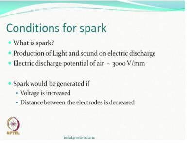
Now, when will it happen? In air approximately discharge will take place to the air if the voltage is or close to 3000 volts per millimeter. So, if there is a millimeter gap and if you have 3000 volt approximately then you will see spark taking place, if the distance is large even at this voltage you will not see, therefore, the voltage are very very high when you have the high tension wires going and still you do not see any spark.
