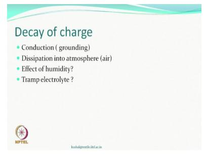
So how can the charge decay well if it touches like you, alighted from a car touch the ground and touch the body of the car suddenly there was a connection and charges would get transferred or if nothing else slowly it can be transferred to the gas the environment also because some charge particles may be there and they can come in contact and some neutralization can take place. Off course as we said if humidity is more, then charge transfer also or decay can take place faster.
