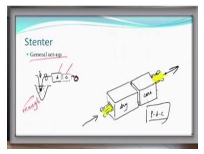
This is done in some general setup like this, you understand this? This is your padding mangle, the wet fabric from here enters a chamber which is called the drying chamber. And then it enters the curing chamber and then of course you can wind it. So, this could be 1 chamber, 2 chamber many more chambers, based on what is the width, what is the GSM of the fabric, what is the expression that you have, how much water therefore you want to remove,
