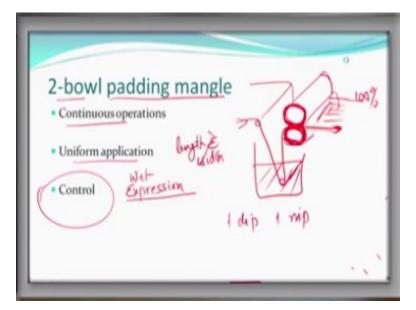
And so, if you use 2, then it is called a 2-bowl padding mangle. So, that we already saw, this is how we pass the fabric in squeeze. So, it is 2 bowl padding mangle. Ok? What is the advantage? It is a continuous process. So, fabric can come from one side, enter, gets merged and then gets squeezed and come out, based on what is the expression, let us say 100% expression or whatever value that you have.
