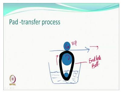
Moving in this direction there will be nip here and you can have an endless belt which can pick up some liquid that side is moving in this direction. This is moving in this direction, this is moving in this direction okay, and show it picks up some liquor depending upon what type of material what is the thickness the amount of liquor can be controlled and then it just transfers only whatever it has picked up.
