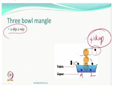
The other mangle that we know is called the 3 bowl mangle which we have seen it got a 2 dip 2 nip situation one dipper second dipper and 1 nip and second nip okay this is how this mangle padding mangle works. Obviously 3 bowl mangle is used when the fabric got high GSM thicker material you are not very sure that one nip would be able to do the job. So you got 2 dip and 2 nip and you got uniform treatment at the end of this you will measure your wet pickup you okay.
