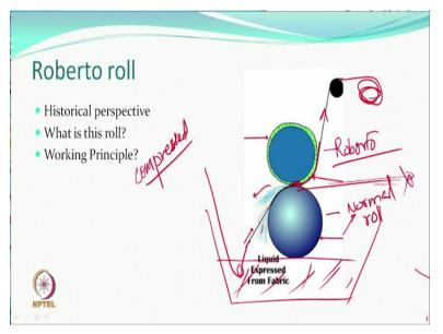
There is another important thing which is developed which is which can absorb more moisture that means a fabric which is been nipt and got certain amount of liquor can something more be taken out that is what is there. So in the pad transfer we try to apply less in this 3 ball mangle system where we redirect the fabric from different ways we are looking at the transfer but removing the water more from the fabric because the other fabric which was dry is also absorbent.
