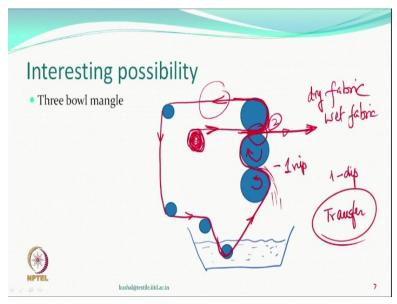
See what was the problem with the bad transfer is that lets you have applied a particular type of a chemical. This belt so called belt can get contaminated because it may absorb because it must be a bit absorb absorbing type material. So some of the chemical will remain and so if you want to add another chemical different chemical industry then some contamination could be seen which one limitation which people may not like okay is.
