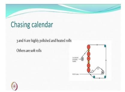
That means the fabric is chasing itself, right? So when it comes in contact with the area, which is a polished surface in this whole sequence roller, all the balls number 3 and 6 are highly polished, and they are also hot. Okay, so that is one part, but the fabric is threaded in a manner that it goes from this side all along goes all the way comes on and then come so at some point there are 2 fabrics coming contact.
