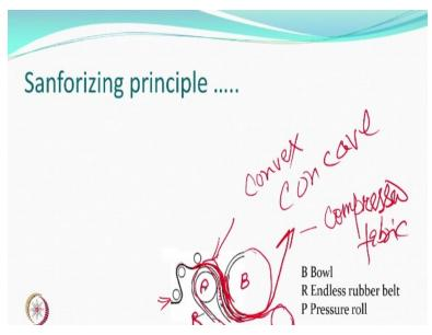
So, this finish is a sanforizing finish, where what we are doing is that you pre shrink the fabrics uniformly. So, that excess length of yarn is available so that when it swells, it does not shrink further because you have already done the compressor shrinkage before. This type of a thing is called the sanforizing processes and sanforizing finish, it obviously shrinks the fabric little bit. So that finally done shrink.
