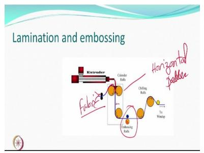
For example, a system where you have a fabric and a polymer which is being excluded as a let us say a molten polymer is coming. This is a horizontal padder kind of a situation. Right. So, what happens is this fabric is coming from here. And the polymer is also coming here and they get in a way come in contact. So, if the fabric is touching the first roller, only one side of the fabric will come in contact with the molten polymer which will get deposited.
