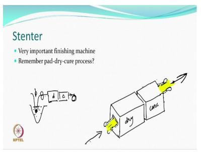
Which is the most important machine in the finishing system. If you remember pad dry cure process, so after padding, the drying and the curing takes place in this machine not on a drying cylinder or not on a festoon. Right so this is if you do pad dry cure of a process like the raising finishing is this is the machine, philomel tendency this is the machine. So, when you do the finishing process this is very important machine.
