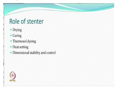
So, the role of the stenter is drying of course, curing yes thermosol dyeing if you had disperse dyeing can be around dyed by a thermosol process at higher temperatures, this type machine will work heat setting we talked about will be done on a stenter the cause it gives you dimensional
