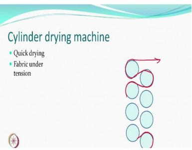
So quick drying this is the type of machine which required the fabric remain under tension you know so that it touches the surface of the cylinder all the time so it would be under tension. If
