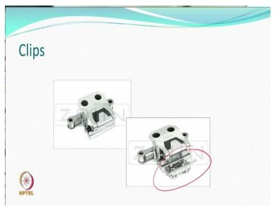
So there are if you do not want the pin marks then there are clips which just hold the fabric and then pull. And sometimes they are combination hybrid kind of system where it is a clip as well as pin system, whichever you want to use, one can use all these type of things will be part of, let us say, stenter, but it is a very sophisticated machine also other than drying and thing because it must sense the salvage correctly. And then pears the pin or clip hold by a clip right.
