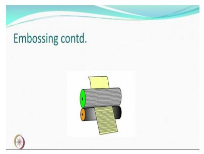
So, if the design is of this type you will get fabric which has got some design of this kind. So, this is what it is whether this effect is going to be temporary or permanent depends on what have you done. If suppose, along with this you have a polymeric system also moving along and with the embossing maybe you can create more permanent effect. Otherwise it can be temporary or you have resin based system which can be cured after this.
