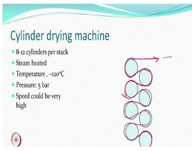
So somewhat simple drying systems are we will just talk about cylinder drying machine so cylinder drying machines there are stacks of cylinders right.? Where the fabric is threaded right goes like this is goes like this goes like this and up to this point and goes out and these are heated by steam and all the cylinders are heated by steam fabric is in contact with metallic surface and so heat is transferred from the metal to the fabric and the water evaporated all over alright.
