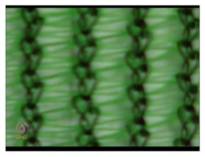
So, here also if you see, if you carefully see, so 1 loop is made from the black yarn and the other loop is made by the green yarn. So, 2 yarns are being catched at the same time, so in the same course. So, each needle is carrying 2 yarns simultaneously, so this is what this structure is showing to you.
