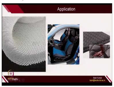
Warp knit fabrics more advanced version is used in car seats also where this is a spacer fabric, we call this in the market 3-D spacer fabrics, again a warp knitted structure, very good cushioning effect and this is again made by warp knitting technologies.
