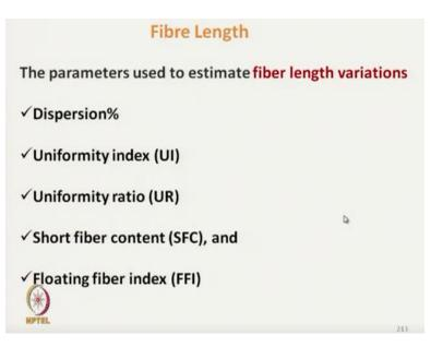
So, length variation if we want to know it is very important for any composite manufacturing, we must know the fibre length variations. So, variation, fibre length variation is dispersion percentage, uniformity index, uniformity ratio, short fibre content, floating fibre index.
