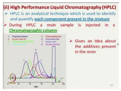
HPLC, so by high performance liquid chromatography, we just we can identify and quantify each component present in the mixture, if we take the mixture or if we take any polymer, so, where whether there are any mixture or not that we can identify using the HPLC. ,t gives an idea about the additives present in the resins. So, what are the different additives present that we can identify.
