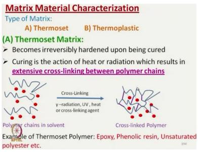
So, you know there are 2 types of matrix materials, one is thermoset, and next is thermoplastic. Most of the characterizations of thermoset and thermoplastics are similar apart from a few additional tests for specifically for either thermoset or thermoplastic, as we know thermoplastic, thermoset matrix, they are irreversible hardened upon being cured during curing action, extensive cross linking takes place.
