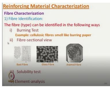
First fibre, I will go quickly because we all this characterization we know. So, we are not going to spend much time. So, fibre identification by a burning test or by fibre solubility test. This we can identify the fibre what type of fibres are there, whether it is a natural fibre, synthetic fibre, cellulosic fibre, so that we can identify the fibre.
