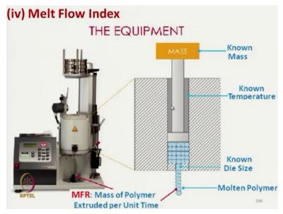
This is the standard equipment. Known mass of material is placed here with a known temperature, known die size and molten polymer, we can measure take the volume or take the mass of the polymer extruded, we can take. Next is that reinforcing material characteristics. So, after matrix we must understand the characteristics of reinforcing material.
