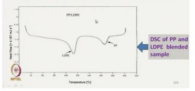
And also from DSC, we can get an idea about the purity of the material. If it is the polymer is pure, then we will get a single peak. But in case of mixed impure sample, the polymer will show the multiple peaks like here example, PP and LDPE, the mixture it gives 2 peaks.
