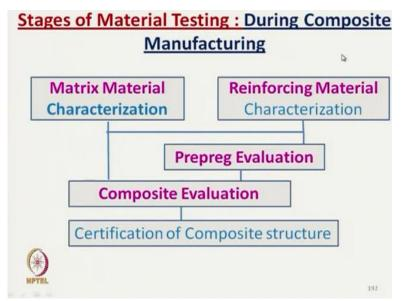
So, the stages are for manufacturer of composites, their raw materials are matrix materials and reinforcing materials. So, first they have to test matrix whether these matrix are as per the specification or as per the requirement. Then, we have to understand the characteristics of reinforcing material. So, we need to test the reinforcing material before we go for the composite manufacturing.
