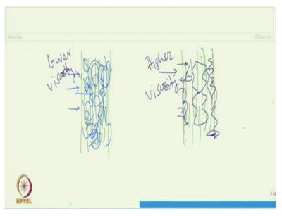
So, let us see, suppose this is the reinforcing structure, this is another reinforcing structure. Now, this is a polymer with lower viscosity, they will penetrate easily inside the structure and with the higher viscosity if we take, so, this is higher viscosity they will not be able to penetrate clearly, so there will be void created within the structure they are not able to penetrate properly.
