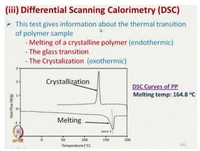
So, DSC differential scanning calorimetry is used for measuring the melting point. (**Refer Slide Time: 18:03**)
