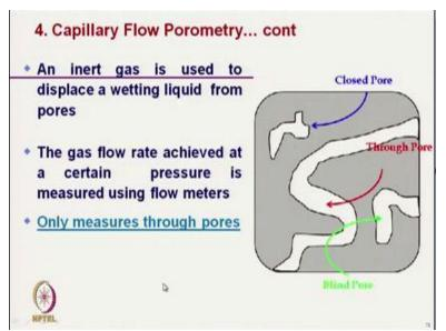
So, here capillary flow porometry the principle is that an inert gas is used to displace the wetting liquid from pores, the gas flow rate achieved at certain pressure is measured using flow meters. So, one full flow meter will be there. So, at certain pressure, we measure the gas flow rate and in this principle we measure only through pores, pore dimension of through pores which are important.
