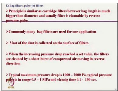
Next is that bag filters. So, the principle wise this is similar to the cartridge filter. So, if you assume that the size of cartridge is very big, then we can conceptualize the bag filter so, let us see the cartridge filter here.
