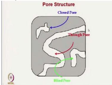
There are 3 different types of pore structures. One is closed pore, which is blocked from all the sides, blind pore its open from one of the surfaces and it ends within the structure and through pores that is the pores are that starts from one surface and ends at other surface. So, this through pores are basically important for filtration application.
