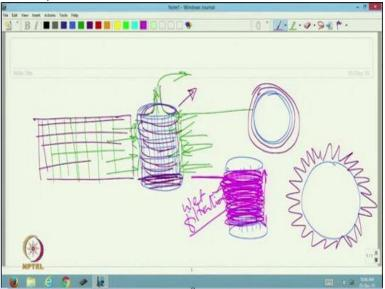
So we need 1 perforated frame for this and in this part this is perforated frame this is only for support. This can be metal mesh or maybe polymeric cylinder hollow cylinder with mesh. Now, on this we can wrap the filter fabric. So, we just wrapped the, this is the filter fabric it could be non-woven, woven, so, this is the filter fabric. So, if we just simply wrap around this and this will be effectively the cartridge filter and one side is blocked and other side is outlet is there.
