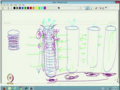
So cartridge filter what we have seen this is the cartridge and we wrap the filter fabric. This is a filter fabric but in case of bag filter we have larger size of frames very large frame. This is a metallic mesh. This is used just for support and the prefabricated bags, filter bags are used these bags are taken here and just placed over this, this is bag filter. This frame is only for support of the bag and frame is required otherwise the filtration process is not possible.
