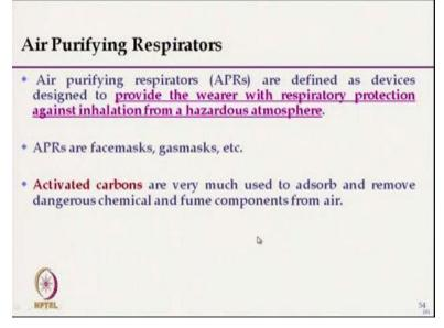
Next filtration is that air purifying respirator, this filters are defined as device designed to provide the wearer with respiratory protection against inhalation from hazardous atmosphere. So this is used for respiratory protection. The examples of APRs are facemask, gasmask. Activated carbons are used to adsorb and remove dangerous chemicals in addition to the particle filter or fumes in the air.
