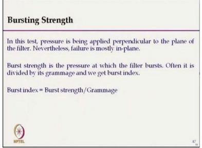
Busting strength is also very important particularly for filter fabric act when the pressure difference that is pressure drop is high. So it is measured based on the diaphragm type busting strength tester, so bust index is measured, which is actually busting strength per unit mass. Now, we will discuss different types of products which are available commercially. As far as the shape, we can divide the filter fabrics in different classes. These classifications are first flat filters.
