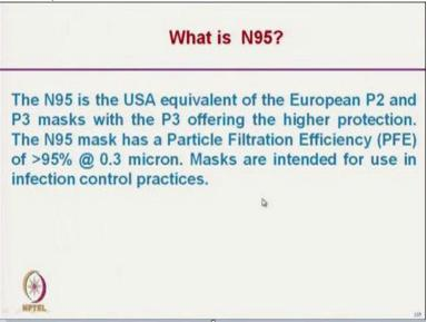
What is N 95? N 95, it is used in US. So, US standard N 95 mask, which is equivalent to European P2 and P3 masks with P3 offering higher protection. The N 95 means it is a particle filtration efficiency more than 95% with the particle size of 0.3 micron. So that is the standard
