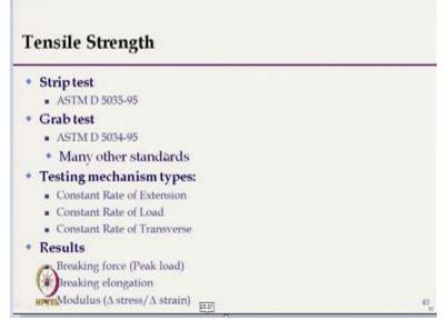
Tensile strength characteristics, they are required. So, strip test, grab test. So, these are the different tests available. So, results are breaking force breaking extentsion, modulus. These are important because during application or handling we must know the tensile characteristics of filter fabric.
