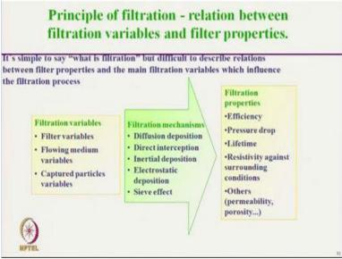
So, after understanding different types of filters based on their shape the relationship between filter variables and filter properties, this understanding it is extremely important for application. So, the filtration variables is that first is filter variable. So, for any filtration we must know what is the type of filter? What is this mass per unit area thickness, what type of fibres are being used, whether it is a head sealed or needle punched, whether it is woven or nonwoven.
