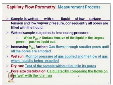
The process is that as I have mentioned here, the sample is first wetted with a liquid of low surface tension. So, that it gets wet easily and consequently all the pores are filled with that liquid. The wetted sample then is subjected to increased pressure of an inert gas. When this pressure of gas P gas exceeds the surface tension of liquid in the largest pore, it will start pushing out the liquid.
