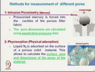
The techniques are, one is intrusion porosimetry that is mercury it is used mercury. So, here mercury at high pressure is forced into the cavity of the porous filter fabric. So, here mercury is being forced through this cavity and depending on the pore structure or pore size the pressure will vary. So, for finer pore size, we need higher pressure. So, poor dimensions are calculated using penetration pressure data. So, indirectly we can calculate the pore dimension.
