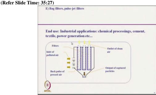
This is a dust collecting system. These are the filters here the dotted line the frames inlet of polluted air and this is a clean air.
