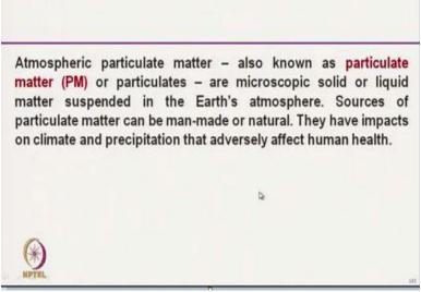
So, if we want to use the filter or APR, air purifying respirator, we must understand the particulate matter in the atmosphere. So, atmospheric particulate matter which is also known as particulate matter, these are microscopic solid or liquid metals suspended in the atmosphere, they are sources are different, maybe natural source or manmade source, but this particular methods are actually harmful for our health. And we must arrest this particular matter from entering into our body.
