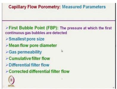
So, this is the pressure at which the first continuous gas bubbles are detected. So, if the pore size is more, this pressure will be less. So, from there we can get idea about the pore size, smallest pore size, mean flow pore diameter, gas permeability that means, when we use the dry run from there we can get to the gas permeability, cumulative filter flow, differential filter flow and corrected differential filter flow. So, these are the parameters we can get from the porometry result.
