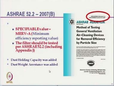
So, there is a parameter which is called MERV Minimum Efficiency Reporting Value as I have mentioned. So, this is one, this is the American system of grading the filter. MERV value source the filters and efficiency. So, dust holding capacity was added in ASHRAE 2007 dust weight arrestance was added.
