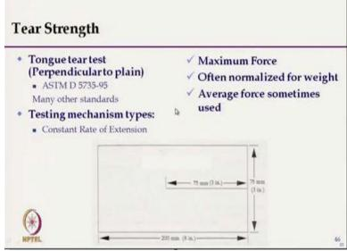
Tear strength is also important, tongue tear strength. So, testing machine any constant rate of extension machine can be used. So, here maximum force, average force of the tear strength sometime used. So these are the parameters which we can use for tear strength the measurement of filter fabric.
