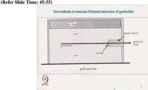
So, here the geotextile is confined in between the soil in both the sides. So, it then pulling force applied and depending on the fictional interaction, the pulling force will change so, from this pulling force we can calculate the interaction between the geotextile and soil.
