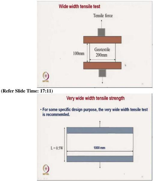
This is the test this the diagram shows the dimensions 200 millimeter and 10 millimeter, for very wide width, the dimension is the width is 1 meter and the length is half of the width. So, this is some time recommended for geotextile application.
