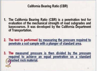
Now, coming to actual CBR, CBR testing California bearing ratio test for soil particles, it is a penetration test for evaluation of mechanical strength of roads subgrade and basecourse. So, road subgrade strength compressive strength we must know, it is developed by the California Department of Transportation that is why the name is California bearing ratio. The test is performed by measuring the pressure required to penetrate a soil sample with a plunger of standard area.
