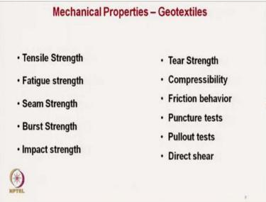
Now coming to mechanical properties, there are a large number of properties. We can test tensile strength, fatigue strength, seam strength, bust strength, impact strength, tear strength, compressibility, frictional behavior, puncture test, pullout test, direct shear test, these are the tests we must perform to get the characteristic to get a clear picture about the performance of geotextiles. So, we will discuss one by one.
