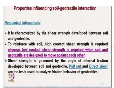
Next mechanical characteristic is that which I have already explained, I am not going to explain here in detail. So, mechanical characteristic is the mechanical interaction, the shear stress is developed shear strength is calculated against the soil. So, it is done by pullout test and direct shear strength test.
