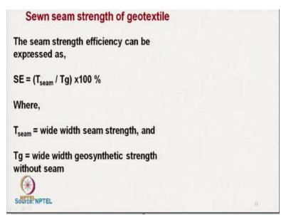
Seam strength efficiency is that the T seam and T strength of geotextile without seam. So, that ratio.
