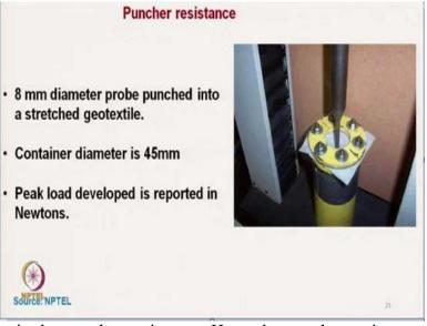
Next characteristics is the puncher resistance. Here, the puncher resistance is measured by 8 millimeter diameter probe, this is 8 millimeter diameter probe and the container diameter is 45 millimeter, this is 45 millimeter here, this is the geotextile material and before just before at or at the time of punching, the peak load is measured and it is expressed in terms of newton and this puncher moves at a certain specified speed.
