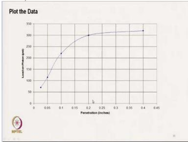
This is the plot we get that is the penetration and the load value or we can get the pressure value. this from this data. This is a plot and from this data we can calculate the CBR value. So let us take 0.1. Here it is 0.1 is coming it is a 220 psi, 0.2 here it is a 300 psi, 0.2 inch.
