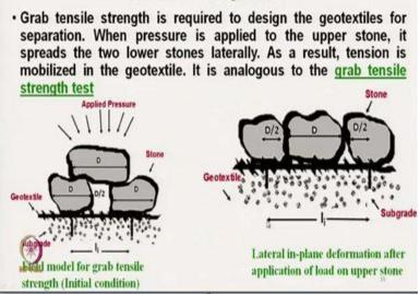
So, this is the diagram. These are the diagrams, the grab tensile strength is required to design the geotextile for separation application. When pressure is applied to the upper stone, it spreads the 2 lower stones laterally, it is trying to spread. As a result tension is mobilized on the geotextile and it is just analogous to grab tensile strength.
