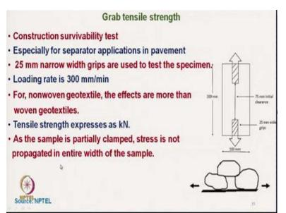
Now, grab test as far as geotextile is concerned, the grab test is extremely important. This is for construction survivability test. Tensile test gives an idea about the mechanical characteristics, but grab test most of the condition the geotextiles are subjected to grab test like situation. In grab test the geotextile material a sample is not gripped throughout the width, it is gripped at center, this situation normally occurs during application.
