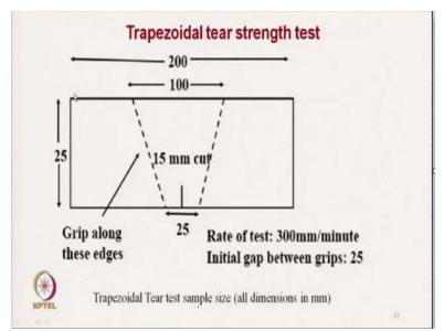
This is the sample size as far ASTM, 200 millimeter length this is 100 and this is the grip line and here the cut is made and we measure the strength required to propagate this cut.
