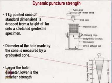
Another parameter which is important is a dynamic puncture strength. This type of situation can occur during laying of geotextile so, where the 1 kg pointed cone is dropped freely on geotextile
