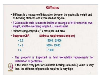
Next coming the important characteristics for geotextiles it is a stiffness. Stiffness as we know, for apparel fabric, the stiffness is important for the comfort characteristics, tactile comfort, or for home furnishing mainly, it is related with the drape, but for geotextile stiffness is extremely important for application with the different types of soil. Now, the measurement techniques of stiffness is similar to that of apparel textile.
