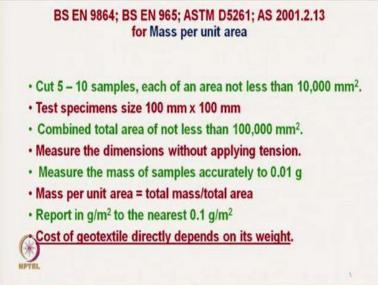
Then mass per unit area is very important, the tensile characteristics mainly correlate with the mass per unit area of material. So, here are the materials are cut in a specific dimension. And the material then is its weight its mass is taken and that when we divide the mass with the area, we get the mass per unit area, while measuring the dimension you should take precaution it should not be stretched.
