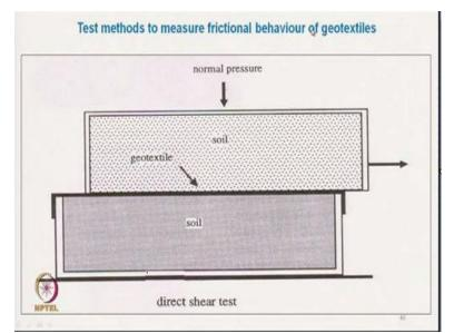
Another method is that it is a direct shear test. Where this is a base soil and top soil is there and on the base soil, there are 2 blocks. On the lower block geotextile is covered with a geotextile and then top soil it is actually slide and it is sheared against the geotextile and we can calculate the shearing force.
