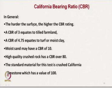
So, if we get the, try to see the standard value CBR value, the harder the surface the higher is the CBR value, a CBR of 3 equates to tilled farmland, very weak farmland, the CBR is 3 and moist clay it is 4.5 and high quality crushed rock CBR is 80, like that and California limestone which is definitely 100. So, as this is the reference value and accordingly we can calculate the CBR value. So, higher the CBR value the stronger that is the rock or the surface will be very hard.
