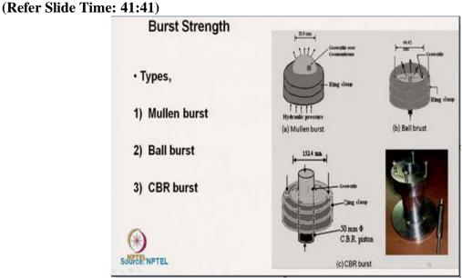
Then another mechanical characteristic which is Mullen as the busting strength. There are 3 types, Mullen bursting strength, ball bursting strength and CBR bursting strength. This CBR testing it is used for puncture resistance also and here we can use as bursting data. So in Mullen bursting strength where the diaphragm is used and ball bursting strength, here one puncher will be used with a ball at the seam and CBR bursting strength is here one plunger with it is a cylindrical plunger is used.
