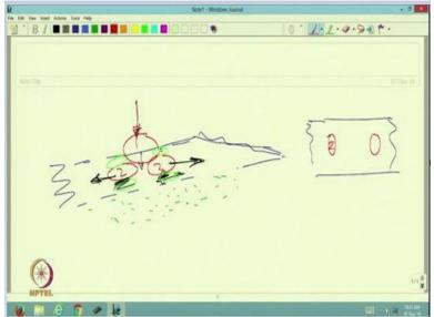
I will show here now here this is a geotextile, this is geotextile. Below that there are soft soils and above the geotextile say this is one stone, another stone this gravel so there now, once the load is being applied on this stone due to the downward force these 2 stones will try to move sideways and due to the contact point and at this point of geotextile, geotextile will be pulled. So, this zones are not being pooled. This is creating one situation.
