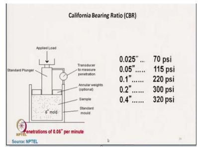
Here if we see that for a given soil we have got a data this data 0.025 inch penetration for that penetration we need to apply 70 psi pounds per square inch. And gradually if we want to penetrate the this plunger at higher distance, we need to apply higher pressure, typically 0.1 inch and 0.2 inch this to data are taken, the pressure required to penetrate 0.1 inch and pressure required to penetrate 0.2 inch is taken to calculate the California bearing ratio.
