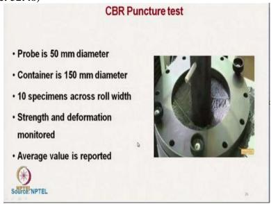
Next punching test is done by CBR Puncture test, the CBR test California bearing ratio test as it is basically for the soil particles, it measures the compressibility of soil. But using this technique, we can measure the puncture strength also, it is similar to earlier test that puncher resistance test where probe diameter was 8 millimeter, but in CBR test, the standard probe diameter is 50 millimeters.
