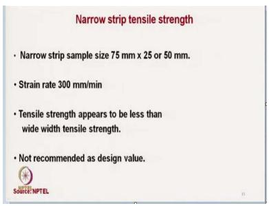
Narrow strip, we can test for just getting the idea, the index value we can get, the tensile strength appears to be less than the wide width tensile strength. As I have already mentioned, this test is not recommended for geotextile design only for getting the idea about the tensile characteristics.
