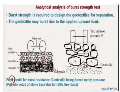
In most of the applications it is actually this type of Mullen bursting strength is used. So, burst strength is required to design the geotextile for separation again, the geotextile may bust due to the applied upward pressure.
