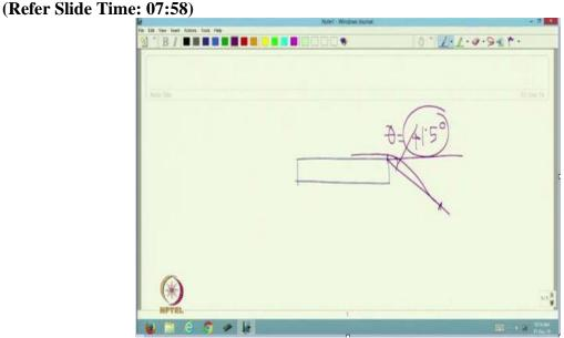
Here the stiffness tester like Shirley stiffness tester can be used the length, overhanging length which is making 41.5 degree angle, that overhanging length is taken as stiffness. So, higher the, this length, higher will be the stiffness. So, 25 millimeter approximately 1 inch wide strip is made to incline at an angle of 41.5 degree and that length is measured and the stiffness value is calculated by this formula that is stiffness in milligrams centimeter is equal to L/2.
