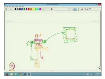
Here this is the heater ok, this is called test plate, and it is connected with the heater, heater 1. Now to prevent the heat flowing in other direction sideway, we want the heat to be flown only in this direction and we want to measure this heat. This is the fabric sample through the fabric specimen, this is what we want, now to prevent the heat to flow sideway direction one insulating material is placed here.
