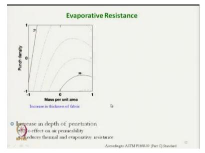
Similar effect was observed due to depth of penetration, it reduces thermal and evaporative resistance and as we see the increase in mass per unit area or increase in punch density, it reduces the thermal resistance, if we increase the punch density, this is due to the fact that as the punch density increases the fabric becomes more and more compact, the air pockets inside the structure reduces, so the thermal resistance also reduces.
