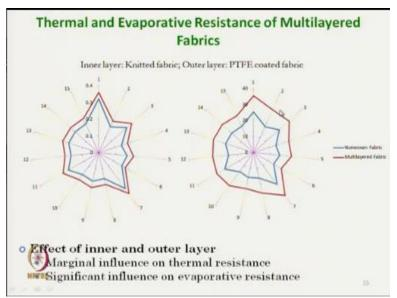
Now in the outer layer if we add inner layer and outer layer, so inner layer was used knitted fabric and outer layer PTFE coated fabric was used with the nonwoven fabric and this is showing the nonwoven fabric with the blue line and the red line showing the multilayer combination. So and this diagram is showing the thermal resistance and in right side it is showing the evaporative resistance.
