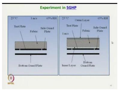
So, guarded hot plate was used for evaluating the thermal transmission characteristics. So this is the sweating guarded hot plate where we can measure the evaporative resistance also.
