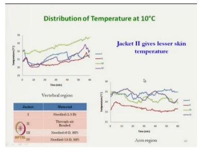
This is temperature is lowest temperature, for other this is much high, so jacket 2 was actually produced through, through-air bonded fabric.
