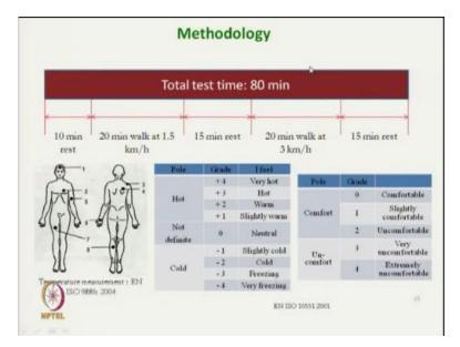
This is the test condition, total test time was 80 minutes, the test protocol here and the subjective assessment was carried out.
