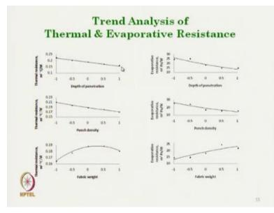
So with the increasing depth of penetration the thermal resistance reduces, as I have mentioned the fabric becomes compact. So this is true for punch density, needle punching density also but if you see the trend for fabric mass per unit area, initially with the increasing mass per unit area the thermal resistance increases, because with the increase in mass per unit area means more fibers are there for resistance but after reaching certain point the thermal resistance drops.
