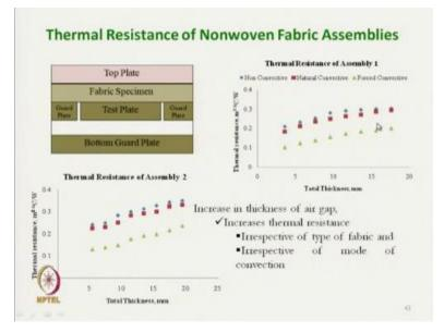
This is the guarded hot plate system where it is bottom plate, test plate, guard plate and fabric specimen and three modes of convective heat transmissions were created one is non-convective mode, natural convection and forced convection. If we do not want any heat to be transmitted through convection if we want to stop convection so, we can use a top plate here so there it will stop the heat transmission through transmission of medium, like air movement is being stopped here.
