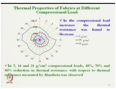
Now the data from this instrument was compared with other standard instruments like sweating guarded hot plate, Alambeta is another instrument for measuring the thermal transmission and this developed instrument and this instrument the minimum pressure available is the 700 Pascal. The thermal resistance of the fabrics, there are different, 20 different fabrics were tested just to understand whether the instrument is giving consistent result.
