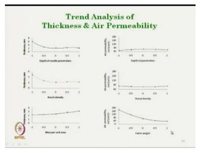
Now if we see the total overall trend as the depth of penetration increases the thickness of nonwoven fabric reduces. Similar trend is observed with the punch density and mass per unit area, as it is increasing the thickness also increases. But the increase in thickness is not that proportion because with the increase in mass per unit area, the fabric compactness overall density of fabric also increases due to more and more entanglement.
