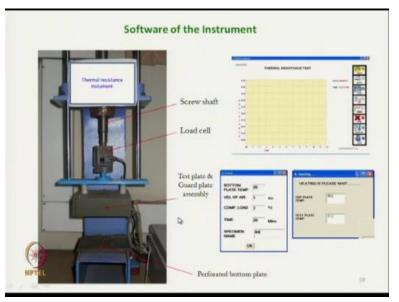
This is the system and this is the photograph of the system the total guard plate system is this is a load cell this is the total guard plate system and perforated bottom plate here and fabric sample is placed here. So we can get load versus thickness curve, as well as a different compression level we can calculate the thermal transmission.
