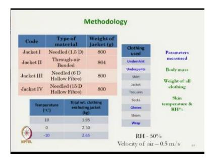
So 4 Jackets were developed, so Jacket 1 the meddler was needled punched fabric, typical mass of jacket was around 800 to 864 within that range. Here inner and outer layers were kept constant for all the 4 Jackets. So Jacket 2 through-air bonded fabric where thickness was very high and this through-air bonded fabric once it was measured in isolation this through-air bonded fabric was having highest thermal insulation.
