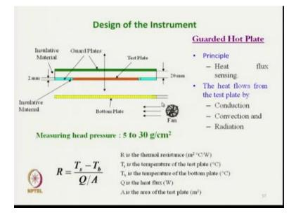
The similar technique was adapted here, but the bottom plate earlier it was it is placed at the top, this is the actual test plate and these are the guard rings, guard plate and the support plate here, which is perforated one and over this bottom plate here the fabric is placed and total this guard ring assembly is connected with the traverse element, where the pressure is applied on the fabric.
