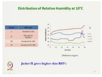
So high humidity is generated and this high humidity is also due to the fact that due to high thickness, very high thickness of through-air bonded. The moisture transmission was not proper. (**Refer Slide Time: 34:03**)
