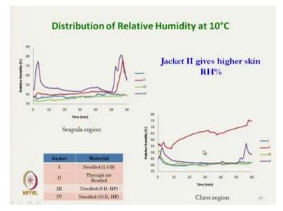
On the other hand if you see the humidity is maximum. So the and the person was feeling cooler due to higher humidity and temperature was low, although this jacket 2 which is made from through-air bonded, it was having very high insulation but once it is coming to the jacket due to higher heat the sweating was there, this is due to sweating, high humidity and that resulted the cooling of the at the skin.
