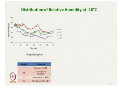
But once we see the humidity again at -10 degree Celsius the layer with very high thermal insulation, it is giving highest humidity at the skin, because the through-air bonded fabric again, its thickness is very high, so the moisture needle transmission does not take place at that rate.
