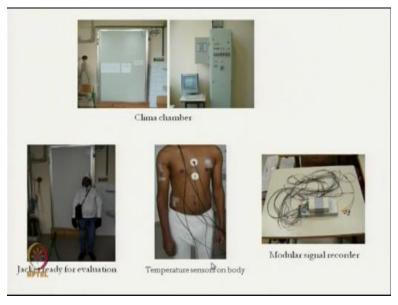
These are the test setup and climatic chamber was there so after wearing this jacket the person entered into the climate chamber.
