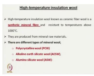
High temperature insulating wool is another type of fiber. They are made from synthetic minerals and resistant to temperature above thousand degree celsius. There are different types of mineral wool, PCW, AESW alkaline earth silicate wool, ASW alumino silicate wool, so there are different varieties of mineral wool fiber.
