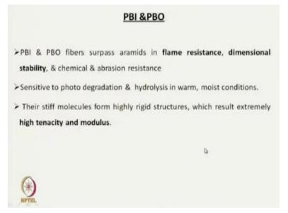
PBI or PBO fibers are used for flame retardant or fire protective clothing. So they suppress aramids in flames resistance and dimensional stability, chemical and abrasion resistance. They are sensitive to photo degradation.
