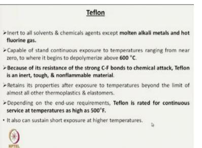
Teflon is another material which is used for fire protective applications.
