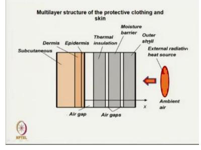
This diagram shows how heat is being transmitted from the source to our skin. This is the external source, this is the radiative heat source there could be flame through the outer layer, middle layer, moisture barrier layer, thermal insulating layer. Heat is flowing and ultimately it is coming to our epidermis, outer layer of the skin and dermis and subcutaneous fat, once the heat is flowing through the layers of fabrics and air gap.
