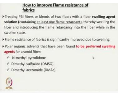
Now if we have a product and we want to improve the flame resistance in the fabric stage, there are different ways to improve the flame resistance. One of the ways is to use swelling agent, like PBI fiber or blends of two fibers, so they are inherently flame resistant and that flame resistance
