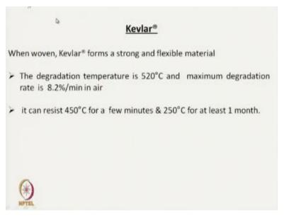
Kevlar is also used so the woven Kevlar fabric is very strong and flexible also as per as degradation is concerned, the degradation temperature is 520 degree Celsius and maximum degradation rate is 8.2% per millimeter in air. So it can resist 450 degree Celsius for a few minutes and at 250 degree Celsius at that high temperature for at least one month it can retain its strength. So at high temperature conditions this fiber is useful. The next material is M5 fiber. (Refer Slide Time: 25:25)
