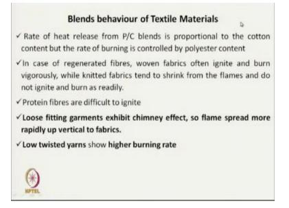
Rate of heat release from polyester cotton blend is proportional to cotton content but the rate of burning is controlled by the polyester. So by controlling the blend or type of yarn we can control the fire, like low twisted yarns can transmit fire quickly. So we use high twisted yarn where air entrapment is less. Loose fitting garments exhibit chimney effect, so flame spread more rapidly up in the vertical direction in the fabric.
