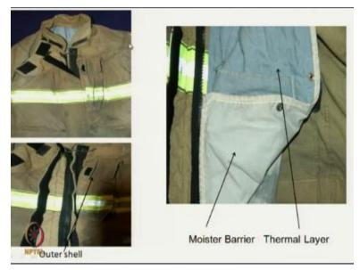
This is the picture of a fire fighting clothing, where this is outer shell, thermal liner, and inner shell and at the middle it is a moisture barrier. So moisture barrier's function is to allow the moisture generated during activity in our body to come out from the inner layer to the outer environment to keep our body dry at the same time it should prevent any liquid, hot water or any sorts of liquid to penetrating inside.
