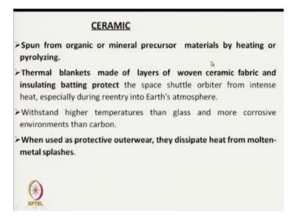
Ceramic fibers are also used, spun from organic and mineral precursor material by heating or pyrolyzing. Thermal blankets, made of layers of woven ceramic fiber and they are used for insulating purpose, so when we use this ceramic fabric as outer layer they dissipate heat from molten material splashes, so we can use ceramic fabric.
