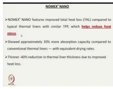
Another fiber, which is Nomex Nano, features improved total heat loss compared to normal typical thermal liner. So which reduces the heat stress, it shows approximately 30% more absorption capacity compared to conventional thermal liners.
