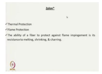
Zylon is another fiber used for thermal protective or flame protective purposes.
