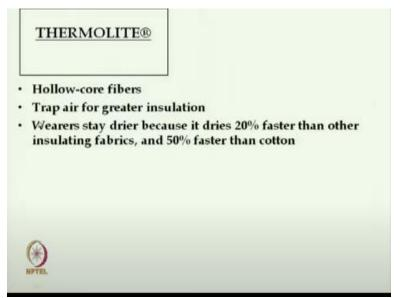
Thermolite is another hollow core fiber. It traps air in the core whereas it is giving insulation. The sports person remains dry because it dries 20% faster than other insulating fabrics. That is the manufacturers claim.
