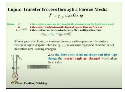
The picture shows here as the fiber cross sectional shape and fiber type changes the contact angle gets changed which actually affect the pressure. So to control the capillary pressure we can select proper fiber and proper fiber cross-sectional shape.
