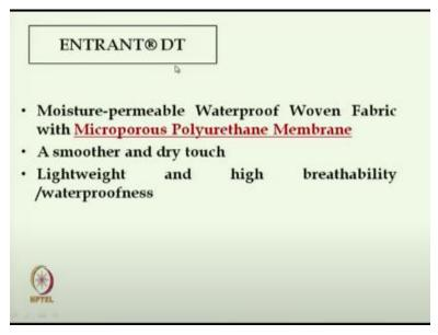
Which is actually coated polyurethane membrane coated; it is waterproof microporous breathable coating on woven fabric. These are smoother and dry touch because it is a polyurethane coating is there and lighter weight and higher breathability and waterproofness, for many application like scuba diving and this type of sports we try to use this type of clothing. Another important characteristics is the anti-static finish;
