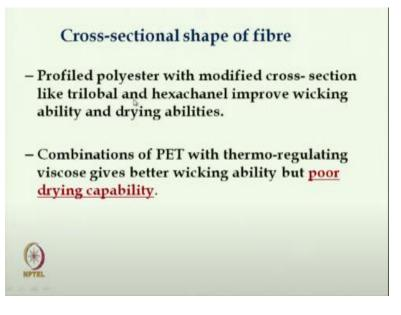
Now coming to the effects of cross sectional shape of fiber the profiled polyester with modified cross section like trilobal and hexachanel improve wicking characteristics. This actually it has been observed that this type of fiber if we change the profile cross section of the polyester from circular to trilobal or hexachanel, it has been observed they are improving the wicking and drying ability.
