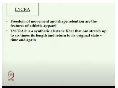
Lycra is another fiber which is basically a well-known fiber. It is an elastane fiber where the high stretchability is there. Freedom of movement, shape retention are the main features of this athletic apparel, so this sportswear the shape in proper form by proper relaxation and due to high elasticity, it adds to free movement of the body. This is a less synthetic elastane fiber and can be stretched up to 600% of its length.
