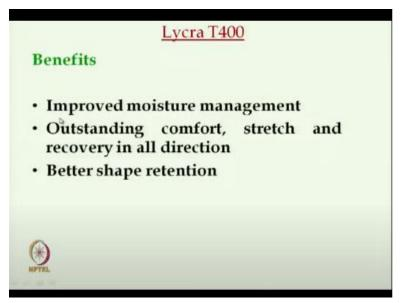
The benefits here is that the improved moisture management so at higher temperature when we need to release moisture at higher rate so due to the crimp formation they will help this pores will help the extra pores help in releasing moisture so enhance comfort, stretch and recovery at all directions and they have better safe retention.
