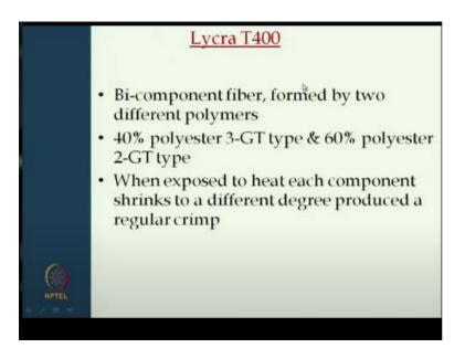
Another special product which is called Lycra T400, it is a bi-component polyester where it is a bi-component fiber from two different types of polymers 40% polyester 3-GT type and 60% polyester 2-GT type. When exposed to heat each component shrink at different degree and which produce the crimp. So the here the phenomena is that;
