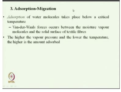
In last class we have discussed the diffusion mechanism, adsorption, transmission, desorption mechanism and the third mechanism of moisture vapor transmission is that adsorption and migration. So adsorption and migration normally takes place for hydrophobic fiber and this phenomena takes place below certain critical temperature and Van der Waals forces occur between the moisture vapor molecule and fiber surface.
