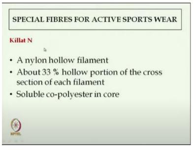
So it can absorb high amount of water keeping the strength and dimensional stability intact. Next is Killat N, this fiber it is a nylon hollow filament about 33% of hollow portion which is produced by soluble co-polyester in the core. So that those cores will get dissolved it is soluble
