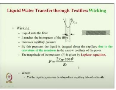
After wetting next is wicking and wicking is followed by this Laplace equation. So this Laplace equation here P is the capillary pressure generated within the capillary between the space within
