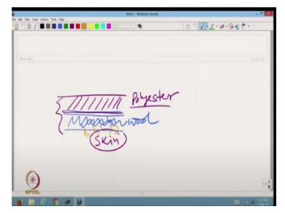
Here in the sports wool this is wool and outer layer is a polyester layer, so two layers wool and skin, our skin. Here whatever the liquid we are generating wool absorbs and from there polyester is that hygroscopic material it takes and wicks to the outer layer that is the mechanism here. It is proposed the polyester draws the moisture from wool and keeps the layer dry.
