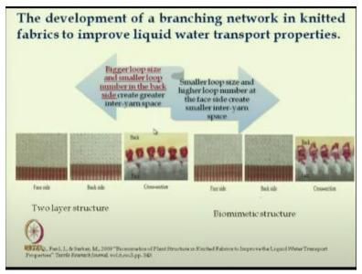
So these are the structures where the bigger loops and smaller loops are created at different layers. So smaller loop size and higher loop number at the face side created the smaller loop size in the size creates the smaller intern-yarn space. So in the face side smaller loops;
