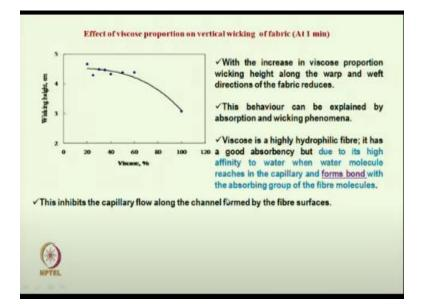
Now here if we see if we take the fabric which we have used we have which we have seen in case of moisture vapor transmission the same set of fabrics we are taking polyester viscose, the viscose proportion is increased from 20% to 100% but here what we have observed here with the increase in viscose content the wicking height, the wickability reduces. The reason behind here the viscous it is a hydrophilic fiber.
