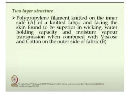
So polypropylene filament knitted fabrics on inner side that is A and the facing the skin this A layer which is made of polypropylene knitted fabric which will be in touch with the skin and it has been found to be superior in wicking because polypropylene wicking characteristics is very high. Water holding capacity and moisture vapor transmission when combination with the viscose or cotton in the outer layer.
