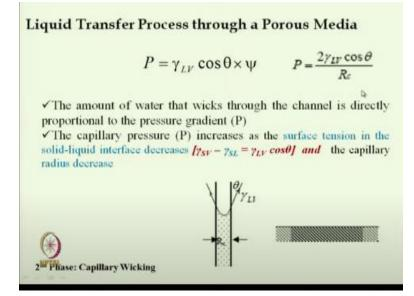
Here it is showing same equation the amount of water that wicks through the channel is directly proportional to the pressure gradient. So that is the pressure here this capillary pressure the capillary pressure increases as the surface tension in the solid-liquid interface decreases and the capillary radius decreases that I have already mentioned so we must engineer our clothing accordingly, sportswear accordingly.
