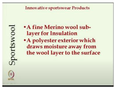
Another innovative product is the sports wool. It is here a fine merino wool sub-layer is used for insulation so inner layer is merino wool layer. Another is the polyester exterior layer which draws moisture away from the wool layer to the surface. Now here we have to see the different products but depending on our requirement we have to use.
