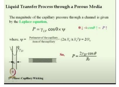
So lower contact angle is higher cos theta, higher capillary pressure that we can do and the Rc is the capillary radius that we can also control.
