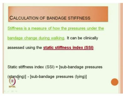
The stiffness is measured is a measure of how the pressure under the bandage changes during walking. So another parameter which we can measure that is called stiffness index. So static stiffness index this will give us idea about the change in pressure during activity. So, static stiffness index; is the difference between sub-bandage pressure in standing condition and sub-bandage pressure in lying condition.
