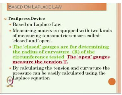
So, one commercial equipment based on this Laplace law is Texilpress device. This works on the Laplace principle. Here as has already been mentioned we need two gauges. So these are basically closed and open. The two gauges are closed gauge and open gauge. The closed gauges are for determining the radius of curvature R of the circumference tested and open gauge is to measure the tension.
