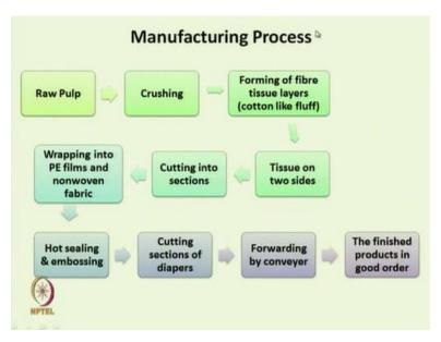
If we see the manufacturing process here, it is a raw pulp; it is crushing, after crushing the forming of fiber tissue layer. So cotton like fluff is produced through the pulp. Then in two sides the tissues are there in the different layers are there, then cutting into section and then wrapped into the polyethylene film and nonwoven fabric and heat sealing and embossing is there, cutting in the form of diaper and then packing.
