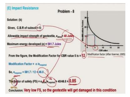
Now, we have we know that CBR value of the subsoil is 5, it is a soft subsoil, that means there will be some modification factor, allowable impact strength of geotextile is 40 joules, so 40 joules is actually it is a allowable impact strength that is the maximum impact sense allowed. So, maximum energy developed as we have seen earlier 561.7 joule that is a maximum energy, now from this modification factor curve by Koerner 2005.
