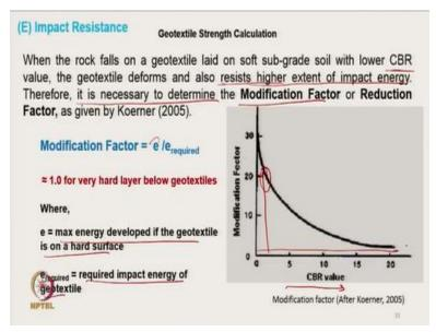
By this is the typical curve here CBR value California bearing ratio value higher the value means the harder the surface. So at lower value so modifications factor is very high that means that effective impact resistance impact energy will be reduced by that that value and it will become typically around 1 for very hard surface. So modification vector is the energy the maximum energy developed.
