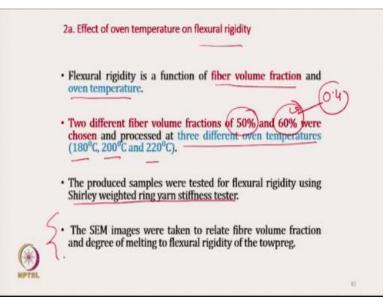
So in this approach we have done other experiments also so we have changed the oven temperature and we have studied the flexural rigidity of the towpreg, so flexural rigidity is a function of fiber volume fraction and oven temperature. So these two parameters we have changed one at a time. So two different fiber volume fractions were taken, 50% and 60%, 60% fiber volume fraction means 40% is the resin weight fraction.
