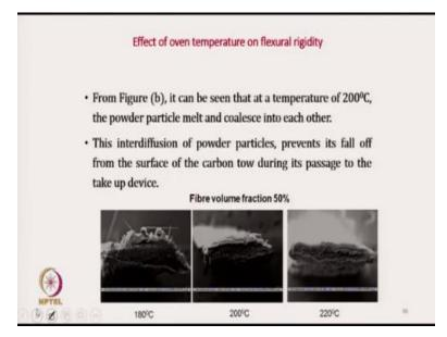
And in figure b this is the figure b which is at temperature 200 degree Celsius powder particle is melted properly and inter diffusion of powder particles were there which prevents its fall off. Inter diffusion is there and at 220 degree Celsius the degree of melting is very high and the reduced reduction in thickness as I have already mentioned.
