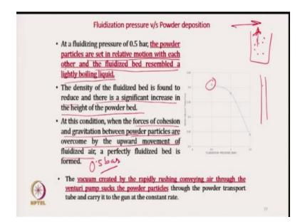
At a fluidizing pressure of 0.5 bar, the powder particles are set in the relative motion with each other which helps in conveying of powder and up to the tow, they set in relative motion with each other and the fluidized bed resembles lightly boiling liquid. The density of fluidized bed is found to reduce; there is a significant increase in height of powder bed. So, that powder bed height will increase that will affect the deposition.
