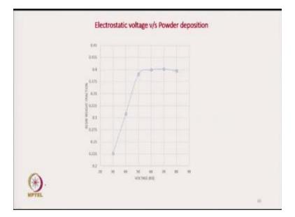
Now the first experiment was done, both voltage was changed the corona voltage was changed and what we have observed with the increase in voltage initially there is a very sharp increase in the resin weight fraction, from say point, 0.225 to 0.4 and after that so after reaching the 50 kilovolt, it is almost stabilized. So after 50 kilovolt, the resin fraction is stabilized, there is no further increase in the resin weight fraction.
