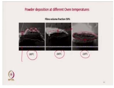
And scanning electron microscope image of the towpreg is there. It is 180 degree Celsius we can see here the powders are not melted properly and it is not deposited evenly but here at 200 degree Celsius this is melted and at further if we can see it is melted and the thickness here at the
