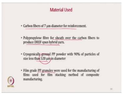
The same material we will be using here the carbon fiber 7 micron diameter and for DREF spinning polypropylene fiber as a sheath will be using on the carbon fibre for producing DREF spun hybrid yarn and for powder coating as the same powder coating principle we will be using with the cryogenically ground polypropylene powder and film grade polypropylene granules were used to manufacture film of certain thickness for film stacking method.
