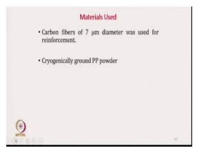
Carbon fiber as I mentioned, we have used the 7 micron diameter carbon fiber and cryogenically ground PP powder.
