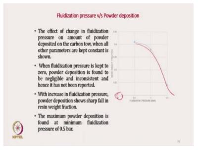
Next is the fluidizing pressure, we have changed here fluidizing pressure from 0.5 bar to 1.5 bar and the diagram shows that it consistently reducing initially at the lower rate and after that it is at high rate, the resin fraction it reduces consistently. So other parameters were kept constant, when the fluidizing pressure is kept zero, so there is no powder generation. So powder deposition is found to be negligible so that is why you have not taken that part.
