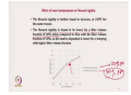
The flexural rigidity is found to be lower in case of 60% volume fraction. So 60% volume fraction, this is the 60%, it is lower. Here the polypropylene, which is responsible for enhancing the flexural rigidity, the content of polypropylene is lower. So 60% fiber volume means 40% is PP, here 50% PP, so due to lower quantity of polypropylene, so that here the flexural rigidity of 60% volume fraction is lower than the 50% volume fraction.
