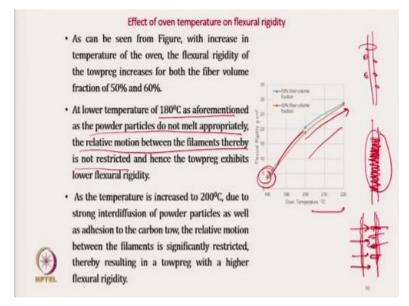
So there is increase, at lower temperature 180 degrees Celsius the powder particles do not melt appropriately. So what happens if it does not melt then there will be relative motion between the filaments. So there is no coating, proper coating, there is fiber, these are the particles. So there will be relative motion between the filaments thereby it is not restricted, the movement is not restricted, so tow exhibits lower flexural rigidity.
