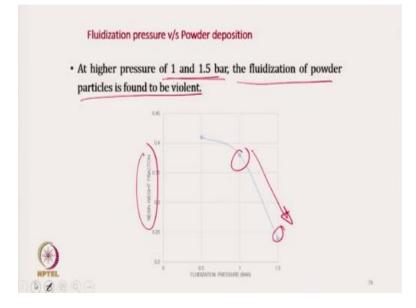
At high pressure, so 1 and 1.5 bar, the fluidization of powder particles found to be violent. So that violent nature is not required and due to this violent nature the powder behaves erratically, the clogging may take place which results in reduction in the resin weight fraction. So for proper deposition we need proper cloud function, it is not that the particle should move violently there should be smooth, light movement should be there.
