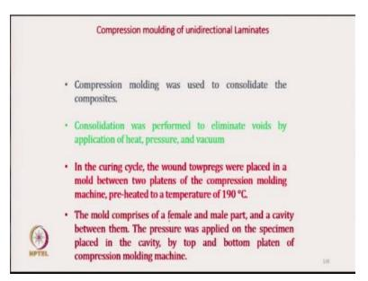
So compression moulding was used to consolidate the composite. So this we have the mould compressor of female and male part and a cavity between them.
