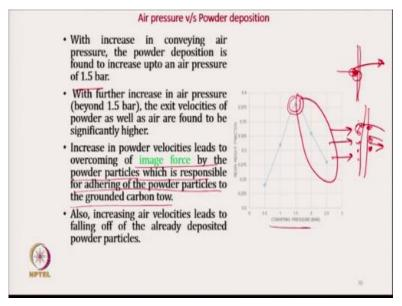
The powder deposition is found to increase up to the 1.5 bar and beyond that significant decrease. The increase in powder velocity leads to overcome the image force by the powder particle, which is responsible for adhering the powder particle to the grounded carbon tow. So initially the powder, the conveying force was required here, so that forces, along with the voltage the powder require some velocity, some speed.
