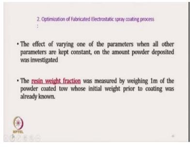
So here what we have done? Here we have changed one parameter at a time keeping all other parameters constant and to investigate the amount of powder deposited on the carbon tow. That is called resin weight fraction and this is done by measuring the weight of the carbon tow before deposition and after deposition, that will give us the indication of the resin weight fraction.
