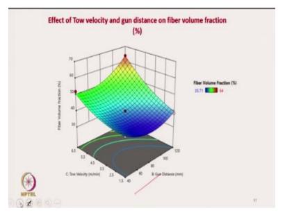
Similarly here this response surface shows the effect of tow velocity and gun distance on fiber volume fraction, so it is showing like as we increase the gun distance here, it is changing. So we can optimize the parameters depending on our use.
