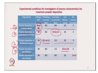
So, these are the different parameters we have used. So here in first experiment what we have done here powder deposition versus corona charge. So here corona charge varies from 30 to 80 kilo volt and rest other parameters like fluidizing pressure, conveying air pressure, gun distance and tow velocity were kept constant. Similarly in the second experiment what we have done powdered deposition versus conveying air pressure.
