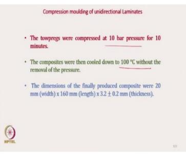
So towpreg was compressed at 10 bar pressure for 10 minutes, the composites were then cooled at 100 degree Celsius without removal of pressure, so pressure was kept and final dimension of the composite was 20 millimeter in width, 160 millimeter in length and 3.2 millimeter approximately it is + -0.2 mm thickness.
