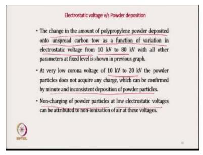
The reason behind this is that the change in the amount of polypropylene powder deposited onto unspread carbon tow as a function of variation in electrostatic voltage from 10 to 80 kilovolt was there when other parameters were kept constant. So at very low corona voltage from 10 to 20,
