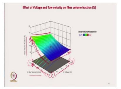
Now, we can see here the same trend that we have got earlier for single variable testing, single variable experiment but here we will get the total response surface. So if we see here the tow velocity, with the increase in tow velocity, the fiber volume fraction increases, means earlier what we have seen with the increase in tow velocity, the resin fraction reduces. It is same, it is with increase in tow velocity, fibre volume fraction increases, that means it is the reduction in resin content.
