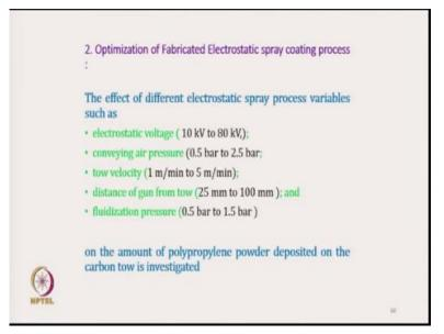
On the resin fraction we will see here the process parameters are the electrostatic voltage this we can vary. So here the electrostatic voltage is varied from 10 kilo volt to 80 kilo volt then, we can vary the conveying air pressure. So, in our study it has the range from point 5 bar to 2.5 bar, other variable is tow velocity. So with the change in tow velocity that is the take up speed, the resin content changes.
