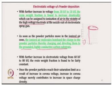
So that is why up to 20 there was no such deposition, with further increase of voltage from 30 to 50 kilo volt, the resin weight fraction is found to increase drastically. As I have mentioned which can be assigned to ionization of air in the vicinity of the high voltage electrode at the nozzle exit point and that helps in that attraction of the particles by the carbon tow. So as soon as the powder particles move in the ionized air zone.
