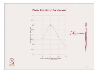
Our next experiment was the effect of distance between gun point gun tip and tow with the powder deposition. So this is the tow and here it is a gun tip. So this distance we have changed. (**Refer Slide Time: 16:39**)
