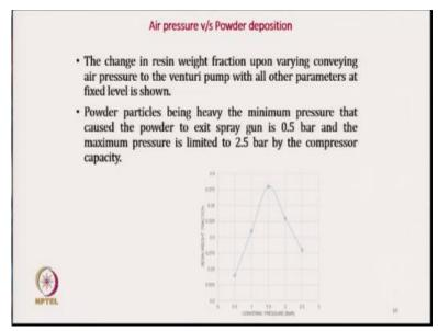
So this is attributed due to the fact that the change in resin weight fraction upon varying air pressure it is basically due to the fact that as we increase the pressure;
