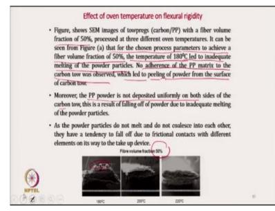
So effect of oven temperature on flexural rigidity if we see so as we have mentioned here, the scanning electron microscope picture with the fiber volume fraction 50% here, it can be seen here that for the chosen process parameters to achieve the fiber volume fraction of 50%, the temperature of 180 degrees led to inadequate melting of the particle, so inadequate melting of the particle.
