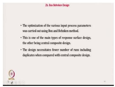
We have used Box and Behnken model, most widely used system.
