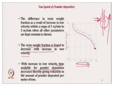
Next experiment was the effect of tow speed on powder deposition. The difference in resin weight fraction we can see with the increase in take up speed it consistently reduces which is basically can be explained by the residence time. If we increase the residence time, then residence time in the chamber, this is the jet gun, powder, if the residence time is more that means more and more powder, will get deposited.
