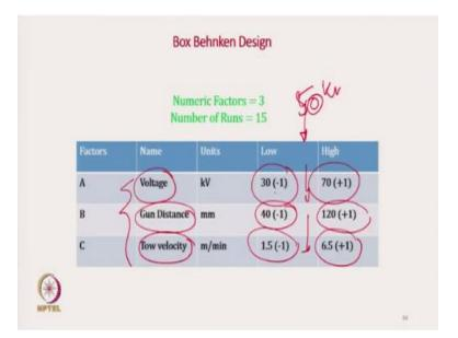
Now here the three variables are voltage, gun distance and tow velocity. These parameters we have seen earlier one at a time but here in combination we have changed the voltage with the lower value is 30 and higher level is 70 kilo volt. Gun distance from 40 to 120 millimeter and tow velocity from 1.5 meter per minute to 6.5 meter per minute and in between at the center value.
