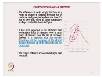
What we have observed initially it increases if we reduce the distance, the deposition is reduced and with the increase in distance, deposition increases up to say 50 millimeter and beyond that if we further increase the distance the resin deposition drops drastically. So from 25 to 100 we have observed here. So it has been reported in the literature that the electrostatic force is strongest at the short distance.
