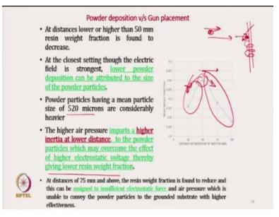
So as the distance is lowered from 50 mm the weight fraction is found to decrease at the closest setting though the electric field is maximum, it is strongest, lower powder deposition can be attributed to the size of the particle. So at that such lower distance, the size of particle is little bit larger, so it has got very high inertia at that inertia if it strikes the tow, it will immediately bounce back or it will not be sticking to the surface.
