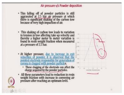
So the falling off is at the further continues with the above 2.5 bar. So there will be shaking action beyond 2.5 bar pressure, so there will be very less resin deposition, okay. So at higher pressure due to increase in exit velocity of powder, it is observed that the pointed electrode responsible for generation of corona it is clogged with the powder particle so at higher pressure it gets clogged. This clogging of electrode can affect the charge acquisition by the powder particle.
