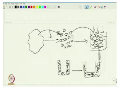
Like if we get, suppose you have one component here, it is a composite suppose it is a used composites. Now we have to grind to make it smaller particle. Normally, we can use a thermoset matrix for using. So this is actually. Then what we do, we mix with this we mix with the polymer. So this is a polymer and there we are mixing with this. After that we will send this to the mold.
