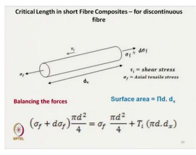
Now coming to the critical length, critical length is nothing but the length which is required, minimum length required, before the when we try to pull that it will below that length the fibre can be pulled out and just above that fibre will be broken before it is coming out from the matrix. So that critical length is important. It is very much important for short fibre composite. And it depends on the shear stress between the fibres and matrices.
