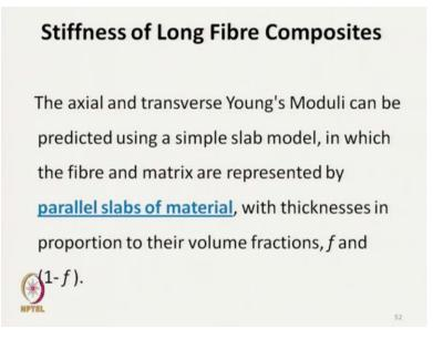
So this parallel slabs of materials, so it has been assumed that the matrix are made of 2 parallel slabs no sorry composite, it is lower portion in green color I have shown, it is a fibre of volume fraction f that is, it is shown by the thickness f and 1 - f is that the matrix. (**Refer Slide Time: 38:04**)
