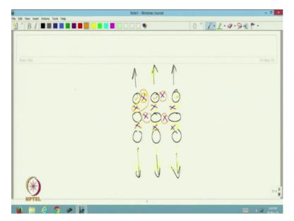
Suppose I am drawing fibres here 1, 2, 3 fibres and 1, ok, now suppose we are applying load in this direction. This is the direction of load, these are the fibres and I am drawing matrix in purple color, these are the matrix in between them. So when the load is being applied in this direction, so this fibre and this matrix, matrix in this 2 positions or this portions this matrices are subjected to a high load because they are in series with the fibre.
