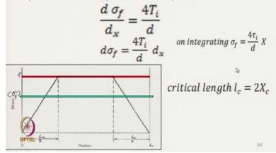
We get this equation, so this is the equation so sigma  $f = 4 \tan i / d$  where and it is X where this X is the critical length.
