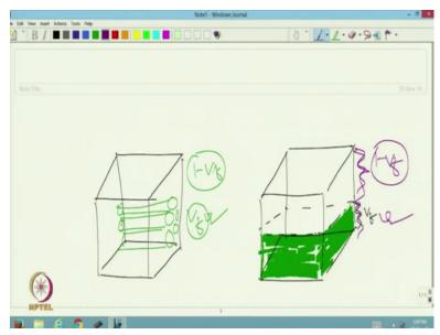
Now let us see what is the model is telling. Suppose this is a matrix, here we have fibres. So fibres are there. Now if we take the actual volume of fibre say V f and total volume is say one volume fraction of fibre is V f so 1 - V f will be the volume fraction of the matrix. So in this model, what we do? We can now, let us draw once again this is the thickness say V f. Now
