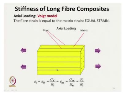
There are 2 models. One is by axial loading it is called Voigt model, another is transferred slowly, I will discuss transverse loading separately. In axial loading, this is the composite block. The black lines it is a fibre, reinforcing fibres and the yellow portion, it is a composite sorry it is a matrix portion. And when these are axially loaded that means the elongation of fibre, elongation of matrix and elongation of the composite they are exactly same.
