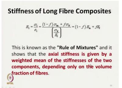
So this is known as rule of mixture. And it shows that the axial stiffness is given by a weighted mean of stiffnesses of 2 components, depending on the volume fraction of fibre. That means if we increase the volume fraction of fibre, if f is increased then the stiffness of the composite will increase because this f this E f is much higher than the modulus of matrix E m, so it is directly proportional to the volume fraction of fibre.
