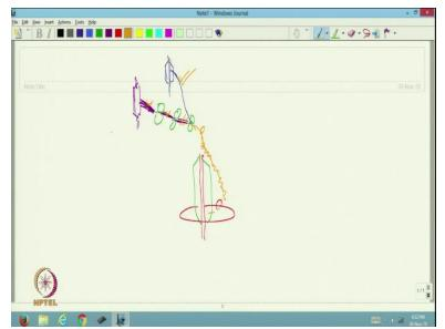
Where these are the drafting rollers and here you have roving of staple fibre, which is actually matrix fibre, and the reinforcement fibre that may be filament or may be staple, reinforcing yarn directly fed to the front drafting roller. From there this form core spun yarn, this is core spun yarn is formed here, where the reinforcing filament or yarn which is not drafted directly is being wrapped by the matrix fibre.
