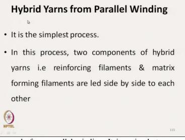
Hybrid yarns are also made from parallel winding. It is a simplest process. 2 components of hybrid yarns that is reinforcing filament and matrix forming filaments are led side by side and wound in parallel form. But here the problem is that the penetration in between the multiple elements of the reinforcing fibre, it is difficult.
