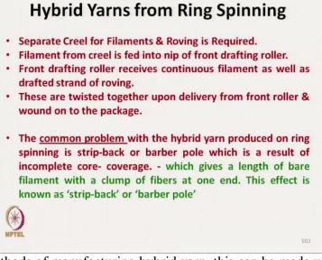
There are various methods of manufacturing hybrid yarn, this can be made using being spun yarn ring spinning process, rotor spinning process, air-jet spinning process, commingling, so there are various processes. In ring spinning we can produce the hybrid yarn using core spun technology. (**Refer Slide Time: 19:31**)
