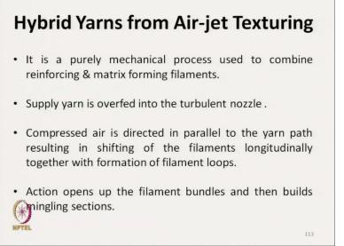
Hybrid yarns are also produced from the air-jet texturing techniques, almost similar process of air-jet spinning, air-jet texturing. Where reinforcing fibre and matrix forming filaments are combined. Similar to commingling process.
