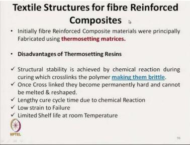
The textile structures for fibre reinforced composites, initially, fibre reinforced composite materials were principally fabricated using thermosetting matrices. The main disadvantages of thermosetting matrices are the structural stability it is achieved by chemical reaction during curing, which is cross linking of polymer. So, that makes the matrices or composite, it is brittle and the transmission is basically permanent.
