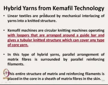
Kemafil, technology is also available where it is a circular knitting machine operating with loopers that arranged around the guide bar and gives a tubular knitted structure which can cover any type of core yarn. So, that here the knitted structure is covering the core yarn and in the core yarn can have both the reinforcing fibre and metrics filament also. But in the sheath it is a matrix filaments are there.
