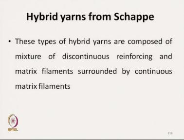
There is another technique; it is a schappe technique, discontinuous reinforcing and matrix filaments surrounded by continuous matrix filament. So that is also one technique of typically it is a type of wrap spun yarn little bit.
