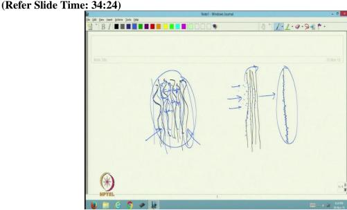
Now, let us see in hybrid yarn what we have seen, suppose this is these are the reinforcing components and these are metrix components. So, we assume that in hybrid yarn matrix component will melt and it will be in between this space of the reinforcing fibres. But we cannot guarantee here that all the filaments will be coated or covered with the matrix component evenly and also there are chances that the reinforcing component this all initially although these are twist less or there is no crimp.
