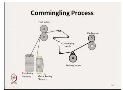
So this is the commingling process, where reinforcing filament and this is the matrix filament. And this is air-jet nozzle where these are mingled together and in commingling these filaments have to be multifilament. So that proper mingling takes place. After that, we can wind and this commingled yarn we can use for converting to fabric or other structure.
