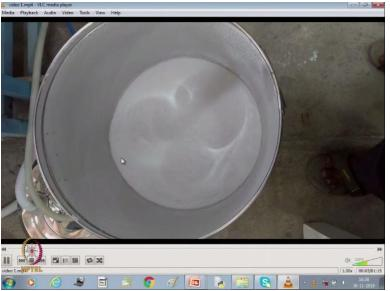
Now let us see here these are the powders of thermoplastic matrix. Now air is being supplied at the bottom, now gradually we will see this bed will become fluidize and the powder will start escaping from that. This is just like it is boiling. So this is and due to the air supplied and while doing this the particles will form cloud. So, as the volume of air increases the bed fluidize and powder particles become suspended, it will start forming the cloud of powder.
