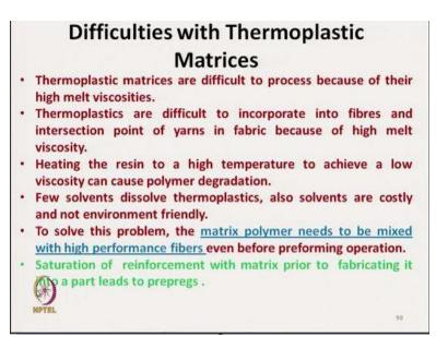
But there are some difficulties. The main drawbacks are, they are difficult to process because they are high melting viscosity. High melt viscosity due to this the penetration within the structure is very difficult. Unlike thermoset matrix, initially their melt viscosity is very low so they can penetrate between the fibre spaces. The thermoplastics are difficult to incorporate into fibre and intersection point of yarn in fabric because of their high melt viscosity.
