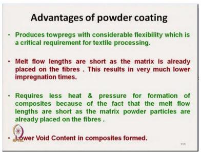
The advantages are produced towpregs with considerable flexibility which is critical requirement of textual processing. So, towpregs basically here are the reinforcement component, that reinforcing filament covered by the powders of the matrix component. So, flexibility is always maintained.
