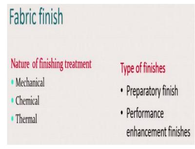
Fabric finishes are categorized based on the nature of the finishing treatments, such as mechanical, chemical, or thermal. The type of finish could also be classified based on its purpose, such as preparatory finishes and performance enhancement finishes. Preparatory finishes are important for improving the dyeability of a fabric.
