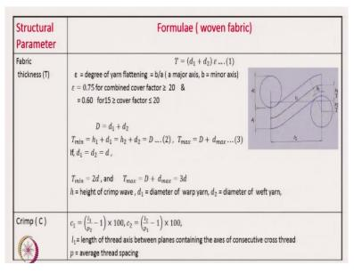
The different types of formulas are stated here, and they must be used whenever required. These formulas are available in textbooks and can help estimate the various design-related parameters. Here the formulas for thickness and crimp are stated.
