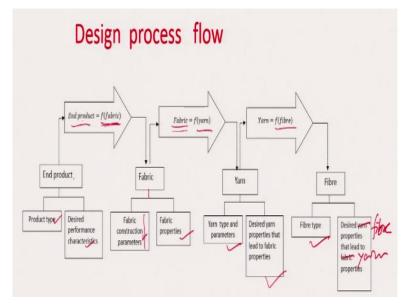
This diagram illustrates the design process flow. Starting from the left-hand side, the process moves toward the right. Typically, designers start with the finished product in mind when they begin the design process. The desired property attributes of the finished product are usually provided, specifying the required performance. Therefore, the first step is for the designer to clearly understand the requirements regarding the product's properties.
