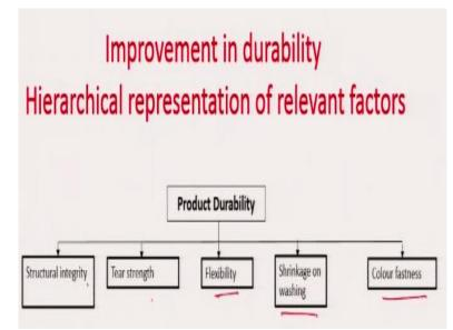
Let's consider an example where durability needs to be improved in a fabric or product. In this case, the designer must first identify the relevant factors that influence durability. These factors can be represented hierarchically to guide the design process. Product durability includes several key aspects, such as structural integrity, tear strength, flexibility, shrinkage during washing, and colour fastness.
