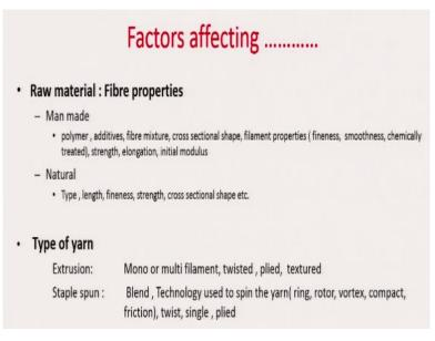
When discussing raw materials, we can categorize them into manmade fibres and natural fibres. There are various parameters of both manmade and natural fibres which affect the properties of the final products. In manmade fibres, the type of polymers used, additives, fibre mixture, cross-sectional shape, filament fineness, filament smoothness, chemical treatment of filaments, etc., have an effect. Strength, elongation and initial modulus are also the parameters for manmade fibres.
