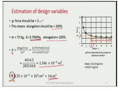
Next is the estimation of design variables, specifically the required area of the rubber cord we need to select. The g-force should be kept below 3 to ensure that it remains within the tolerable limit for humans. This implies that the elongation of the cord must be more than 200%, as shown in the diagram, where 'g = 3' is indicated. Therefore, the elongation region should extend from this point, with a minimum elongation of 200% or greater.
