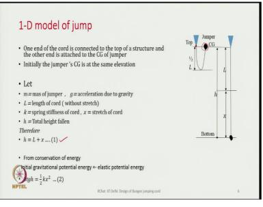
Here, the schematic on the right-hand side illustrates a one-dimensional model of the jump. In this diagram, the jumper is seen, with the cord attached at one end to the jumper's centre of gravity (CG) through a harness and the other end connected to the top of a structure. The diagram also shows the length of the cord, its extensibility, and the total length, including any extensions during the jump.
