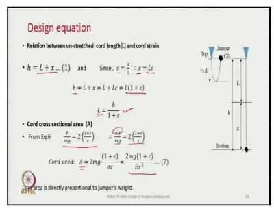
The design equations can be written based on the relation between unstretched cord length and cord strain. It has been seen that 'h = L + x'. Since ' $\varepsilon = \frac{x}{L}$ ', the equation becomes,  $h = L + L \varepsilon$  i.e., the original length of the chord multiplied by strain. Substituting the value of 'x', the length of the cord in an unstretched state is given by ' $L = \frac{h}{1+\varepsilon}$ '. For calculating the cord cross-sectional area, the equation,
