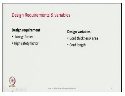
The key requirement for the bungee cord design is to minimize g-forces. High g-forces can be harmful to the individual, so it needs to be ensured that they remain at tolerable levels. The design must incorporate a high safety factor to prevent the cord from failing during use. The primary design variables in this case include the cord thickness, the cross-sectional area of the cord, and the length of the cord that should be utilized.
