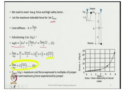
It is necessary to ensure that the g-force experienced during the fall is very low, g-force refers to the acceleration a person experiences while falling and the reverse force they feel because the cord will extend. To meet this requirement, the design must achieve low g-forces and maintain a high safety factor. Let the maximum tolerable force be denoted as ' $F_{max}$ '. The stiffness of the cord 'k' can then be expressed as
