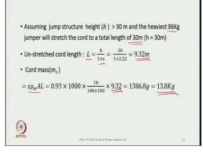
Let us assume that the jump structure has a height of more than 30 m, which is necessary for the person to jump and the cord to fully extend. Given that the total height available is at least 30 m, and the heaviest jumper will stretch the cord by 30 m, the unstretched length of the cord can be calculated. Using the equation for the unstretched length of the cord, it is found to be approximately 9.32 m. This means that the required cord length is 9.32 m.
