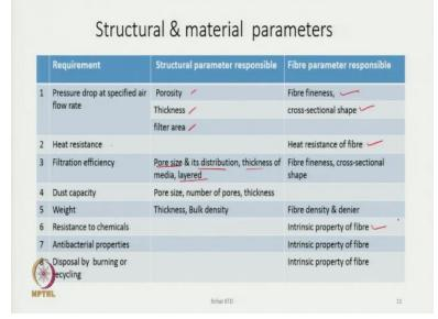
The important structural and material parameters are stated in the table. If the requirement is a pressure drop at a specified airflow rate, the key structural parameters are porosity, thickness, and filter area. For fibre parameters, fibre fineness and cross-sectional shape are important. In this context, the performance criteria, such as pressure drop, heat resistance, filtration efficiency, and others, are linked with the relevant structural and fibre parameters.
