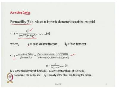
This is another interesting equation related to permeability. The permeability of fibrous media has been the focus of research by many scientists, resulting in numerous complex equations. One equation that is commonly used and found to be quite suitable for initial estimations. It allows us to quickly arrive at practical values, which can help in product development.
