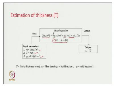
When estimating the fabric thickness, the basis weight is related to the fabric's thickness, fibre density, and porosity. This relationship can be expressed through an equation,
