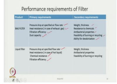
Next comes the nonwoven filter fabrics. The performance requirements for a filter includes several key factors. For a back filter, the most important criteria are pressure drop at a specified airflow rate, heat resistance, filtration efficiency, and dust capacity. Secondary requirements include weight, thickness, resistance, antibacterial properties, the ability to be burned or recycled, and deodorization capabilities. These are the secondary requirements.
