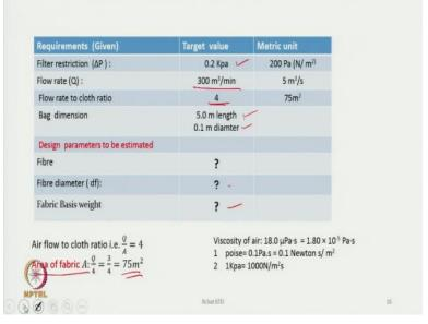
Consider the example of filter restrictions, where the pressure drop is 0.2 kPa, the flow rate is 300 m<sup>3</sup>/min, and the airflow-to-cloth ratio is 4. The bag dimensions are 5 meters in length and 0.1 m in diameter. The appropriate fibre diameter and the fabric basis weight have to be estimated. To begin, we note that the airflow-to-cloth ratio is given as 4. This indicates that  $\frac{Q}{A} = 4^{\circ}$ . Hence, the
