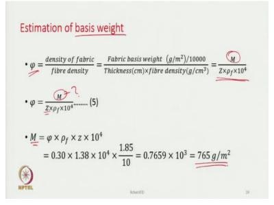
After estimating the thickness, the next step is calculating the basis weight (M). The solid volume fraction is related to the basis weight by the equation
