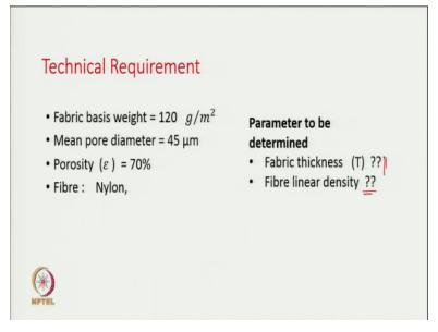
Let's assume the technical requirements specify that the fabric's basic weight should be  $120 \text{ g/m}^2$ , the mean pore diameter should be 45  $\mu$ m, the porosity should be 70%, and the fibre material should be nylon. Given these parameters, we must determine the fabric thickness and the fibre linear density.
