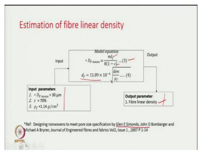
The next aspect is the estimation of fibre linear density. For this, two equations are used. Equation number 3 relates the average pore diameter to fibre diameter and porosity, which is
