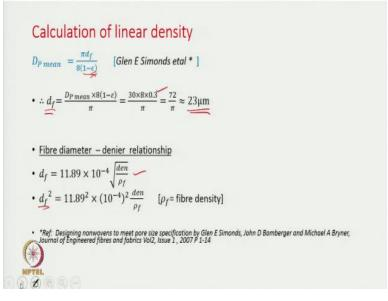
The diameter of the fibre can be determined by using the equation
