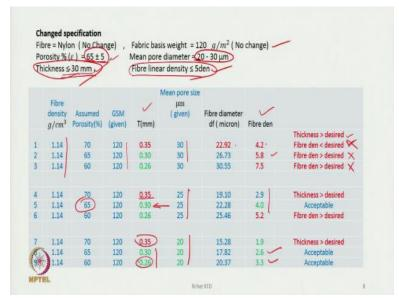
Similarly, in the last set, we must reject the first case because the thickness exceeds 0.3 mm. However, in the other two cases, both are acceptable since the fibre denier is less than 5 and the thickness is 0.3 mm or less. So, there are three valid options: either use 4 denier fibre and make a fabric with 0.3 mm thickness, use 2.6 denier fibre with a fabric of 0.3 mm thickness, or use 3.3 denier fibre with a fabric of 0.26 mm thickness.
