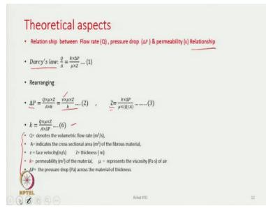
It is essential to know some theoretical aspects when designing filter fabrics, particularly the relationships between flow rate, pressure drop, and permeability. A fundamental equation in this context is Darcy's Law, which states that
