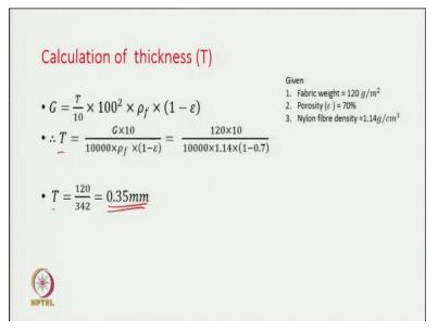
Using the previous equation, where the basis weight 'G' is provided, fabric thickness 'T' can be calculated. By applying the equation, the value of 'T' is found to be 0.35 mm. This means that, in this case, a very thin fabric must be produced with a thickness of only 0.35 mm.
