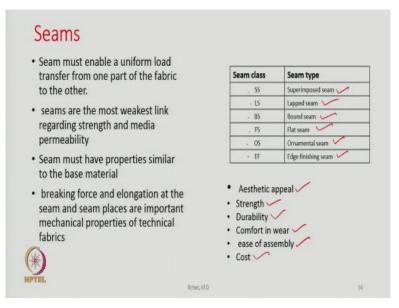
Seams: The seam must enable a uniform load transfer from one part of the fabric to the other. Seams are the weakest link regarding strength and media permeability because there is a chance of perforations during stitching; there is a chance of hole formations. Stitching can also lead to damage to the fabrics. If the stitching is not done properly, it leads to high chances of seam puckering. Anyway, we bring the two fabrics together to stitch them.
