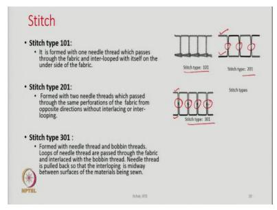
Stitch: there are different types of stitches are shown in the slide. They are stitch type 101, stitch type 201, stitch type 301, etc.; Stitch type 101 is formed with one needle thread, which passes through the fabric and inter-looped with itself on the other side of the fabric, as shown in the figure. So, the needle thread is inter-looping with itself only.
