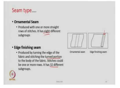
Ornamental seam: they are produced with one or more straight rows of stitches. It has eight different subgroups. Edge finishing seam: if the edges are not properly seamed, the threads may be fraying. So, to avoid such a problem, edge finishing seams are used. It is produced by turning the edge of the fabric and stitching the turn portion as it is shown in the figure. The dotted line indicates the stitch line.
