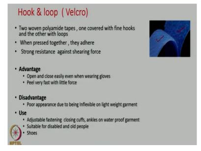
The next mechanism is hook and loop. An example of such a mechanism is Velcro. Most of us are familiar with Velcro. Two woven polyamide tapes, one covered with fine hooks and the other with loops, are pressed against each other, as shown in the diagram. During pressing, they will adhere, and create strong resistance to shear, whereas they offer very little resistance to peeling. The advantages are to open and close easily, even when wearing gloves, and peel very fast with little force.
