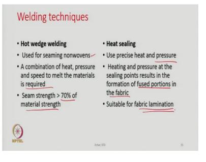
The hot wedge welding technique is usually employed for seaming nonwovens. A combination of heat, pressure and speed to melt the material is required for seaming. Obviously, we cool them to create a joint between the fibres. The seam strength becomes 70% of the material strength in this technique.
