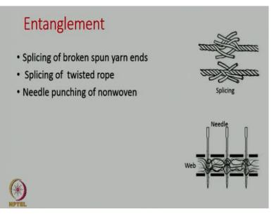
The first mechanism is the entanglement. It is well known that entanglement is a mechanism to join the broken spun yarns using splicing technology during yarn winding. The splicing of twisted ropes is also a kind of joining.
