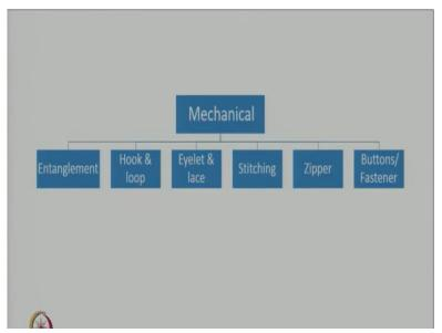
What is the mechanical way of joining? Within the mechanical way, it is further classified based on the mechanism of joining as entanglement, hook & loop, eyelet & lace, stitching, zipper and buttons/fasteners. The joining material may not always be fabrics; the product may be yarn, a braided structure, or a twisted rope.
