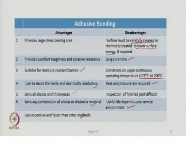
Adhesive bonding: the advantages and disadvantages are listed in the table. The advantages are providing a large stress-bearing area, excellent toughness and abrasion resistance, suitable for moisture resistance barrier, can be made thermally and electrically conductive, joins of all
