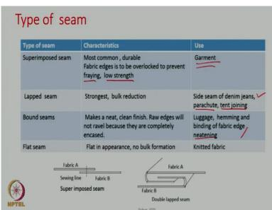
The designer must choose the right kind of seam for specific end-use. The characteristics of superimposed seams are they are most common and durable, fabric edges are to be overlocked to prevent fraying, and they have low strength. They are mostly used in garments.
