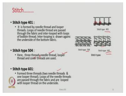
Stitch type 401: it is formed by needle thread and looper threads. Loops of needle threads are passed through the fabric and inter-looped with loops of the bobbin thread. Inter-looping is drawn against the underside of the bottom of the fabric. So here, the inter-looping part is very close to the bottom part of the fabric, so that is how these stitches are made.
