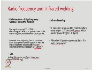
Radiofrequency and infrared welding: radio frequency welding technology uses highfrequency electromagnetic energy to generate heat in the material by virtue of their electrical properties. Normally, it is used for joining films or thin sheets since a strong electric field capable of melting the material can only be achieved when the electrode and the welded part are less than 1.5 mm.
