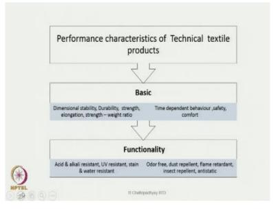
For example, let us take technical textile products. Technical textiles are a vast field, and many types of technical textiles are present, like geotextiles, medical textiles, and many other types of technical textiles. In general, the basic properties of technical textile products are dimensional stability, durability, strength, elongation, strength-weight ratio, and their time-dependent behaviour, safety, and comfort. These are the basic property of the technical textile fibres.
