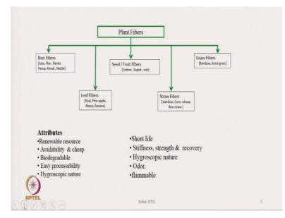
The plant fibre varieties are further classified based on bast, leaf, seed, straw, and grass. The main advantage of natural fibre is that it is obtained from renewable resources. It is also available and less costly. The other biggest advantage is that they are biodegradable, and processability is also considerably easier. They are hygroscopic in nature, which means they have the capability to absorb moisture. Besides these advantages, they possess certain disadvantages as well.
