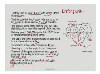
Now, drafting unit 1 if you look at you are already familiar with the drafting system we have studied drafting system on draw frame once roving frame or ring spinning machines and. So, many places roller drafting system most of you have already studied. So, here also we have basically a roller drafting system and we have four pair of rollers because we have to give very high draft.
