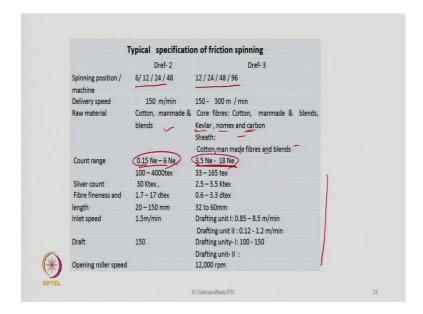
Here is the specification of the friction spinning machine. Dref 2 and Dref 3, spinning positions could be like this. We can get a machine with 6 or 12 or 24 or 48 positions. For Dref 3, it can go up to 96 positions. Delivery rates are also stated here. The kind of fibres it can process. See here, we have fibres in the case of Dref 3, Kevlar, nomex, carbon. They can be there and they can be put into the core. Or sheath, we can have cotton manmade fibres or blends.
