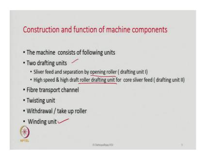
Construction and functions of machine components. So, we have already seen what are the main machine components one is the drafting units there are two drafting unit 1 of them is drafting by opening rollers and the other one is drafting by roller drafting units. Fibre transport channel twisting unit withdrawal or take-up rollers and then the winding unit. So, these are the basic you know components of the machine.
