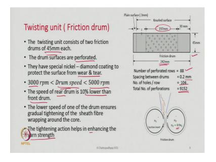
So, here is the simple sketch of the friction drum. Part of the drum surface, almost 197 millimetre in length is having lot of fine perforations. The total length is 242 mm. And the surface of the drum is also knurled. So, that there is a friction. You have to have good friction between the drum surface and the fibre.
