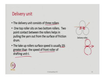
Delivery unit is consist of as it is shown here. Three rollers are there and there are 2 nip zone. This is going to help to pull the yarn at a very very. We have to pull the yarn at a very faster rate know, delivery rate is 180 or 200 or 250 meters per minute. So, just having 2 rollers grip on a yarn is not sufficient to pull the yarn at a very high speed. There is a possibility of slippage.
