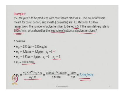
We will take another example what is this example now example number 2 read the example 150 tex yarn is to be produced with core sheath ratio 70 is to 30. The count of sliver meant for core that is cotton and sheath polyesters are 3.5 kilo tex and 4 kilo tex respectively.
