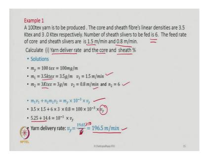
So, now we will solve a problem and that will make it clear problem number 1, or example 1. A 100 tex yarn is to be produced the core and sheath fibre linear densities are 3.5 and 3 kilo tex respectively. Number of sheath slivers to be fed is 6, the feed rate of core and sheath slivers are 1.5 and 1, 0.8 meters per minute. We have to calculate the yarn delivery rate and the core and sheath percentage in the yarn.
