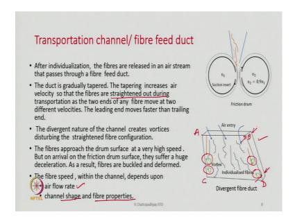
And transport or fibre channel is. So, we have discussed about transport channel also in the while discussing rotor spinning as well. So, here also so many there are more fibres have to be transported power unit time. So, transport channel is little larger and this is the typical you know design of the transport channel that it is divergent in nature. See if you look at the from here to here the distance, let us say I write A and B, if I write C and D. So, C D is larger than A B.
