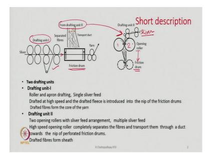
First we will give a very short or brief description of the technology. What you see here is a simple line sketch of the two important parts of the machines. What we see here that there are two drafting unit in this machine. You can see say that this is a basically constructional view of the you know the most important area of the machine not the entire machine as such is basically kind of simple line diagram.
