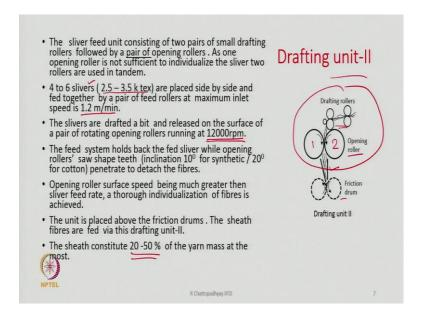
Drafting unit 2 is similar to what kind of drafting units we have in the case of rotor spinning machines where the fibres from the slivers are separated by one opening roller. Here we have two opening rollers 1 and 2 not just 1. The two rollers are required because of complete separation individualization we are actually feeding 5 to 6 slivers or 4 to 6 slivers are fed.
