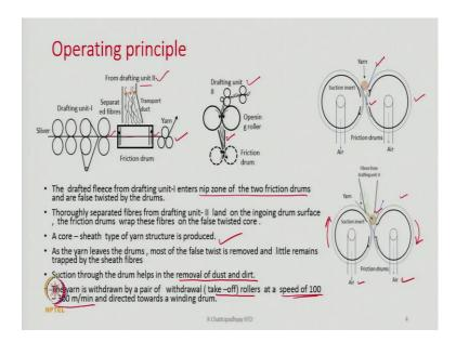
So, that is the direct basically description of the machine in simple terms and if we want to understand the how the machine works then as I said earlier the drafted fleece from the drafting unit 1 will enter the nip zone of the two friction drum. So, here it is shown that this is the nip zone and a bundle of fibres which is existing here shown by the orange colour this bundle of fibres is actually the set of fibres which are being fed through drafting unit 1.
