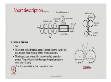
This side of the diagram there are two friction drums drum number 1 and drum number 2 the friction drum surface is perforated. So, there are lots of perforations on it and then there are two suction insert here this you know this circle that you see which is partially opened over here this is basically an insert inside the drum. So, on both side of the drum we have two suction insert and these inserts are connected to a suction pump.
