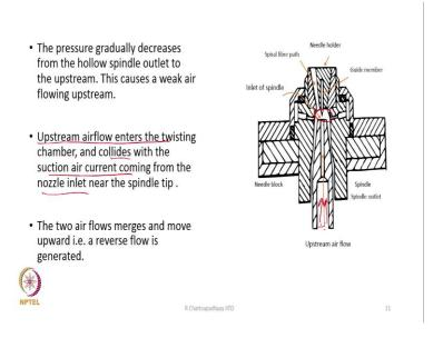
The pressure decreases from the hollow spindle outlet to the upstream; this is another interesting part of it that from here to upwards, see this is the hollow part of the spindle through which the yarn is running. But the pressure at the bottom is more than the pressure at the top within the hollow part. If there is a pressure difference, the air is going to move towards the tip of the spindle.
