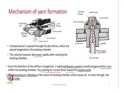
Now, we will give little more attention to the yarn formation, the nozzle block is the heart of this vortex spinning system. Compressed air as it is passed through this jets this jet or you can this side this is the jet. The velocity near the jet is going to increase, because it is very very narrow.
