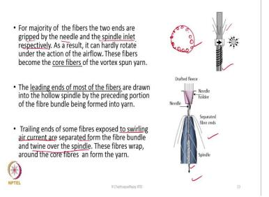
So, for majority of the fibres the two ends are gripped by their needle and the spindle inlet respectively. As a result, it can hardly rotate under the action of the air flow, most
