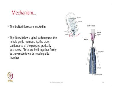
Because of this negative pressure the suction the drafted fibres are sucked. So, drafted fibres know is not going here and there once they are you know moving out of this front roller nip, they are automatically coming towards the inlet that is a nozzle inlet.
