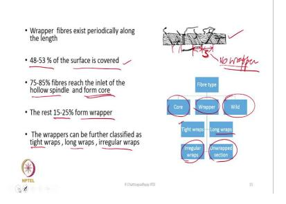
Now, there is another classifications where fibre type has been classified in the yarn as core fibres, wrapper fibres and wild fibres. And wrappers are being also classified as tight wraps the nature of wrap, by wrapper we mean simply wrapper, but then the wrapper fibres can be further classified as tight wraps, long wraps and irregular wraps.
