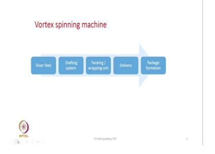
So, today we are going to discuss Vortex Spinning, in the vortex spinning machines what we have is a sliver feed system which is generally a can and this will be followed by a drafting system. And then we have a twisting or you can say wrapping unit followed by this unit we have a delivery, because by the time we have formed the yarn through twisting and wrapping actions the yarn has to be delivered.
