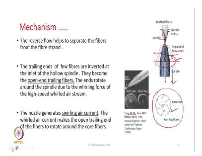
So, the leading end is actually inside they are part of the yarn, the yarn trailing end is existing somewhere here. But the trailing end of the separated fibres have started swirling around the spindle, because the swirling air current exists here. The swirling air current which is surrounding the spindle it has been generated by the jets and they are going down and down the swirling air current.
