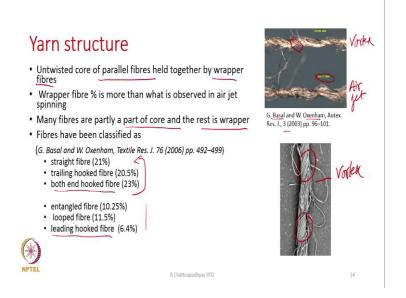
Now, we will discuss the yarn structure, if you look at the yarn structure is a comparison this was done by Basal and Oxenham one paper, this is the air jet yarn and this is the; so, this is vortex and this is air jet, this is also vortex. So, you see that these are the fibres which are wrapping; here, these are the fibres which are wrapping. So, typically the yarn structure is like this untwisted core of parallel fibres held together by wrapper fibres.
