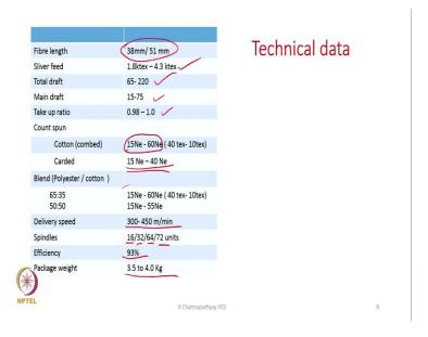
Some technical information about the machine fibre length which it can process easily is 38 or 51 millimetre in this range, sliver counts is given also 1.8 kilo tex to 4.3 kilo tex. So, fibres a little finer side or the total draft we have already said it is 65 to 220 that is the range in some machines.
