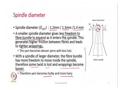
Now, spindle diameter. So, this is the spindle. So, this is the spindle diameter is shown here. This diameter of the spindle. This is hardly 1.2 mm or 1.3 mm or 1.4 mm. And within this diameter also there is a hole, through those holes the fibres are passing. So, you can imagine that you know how small these holes are.
