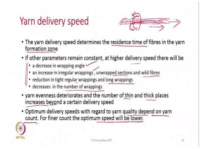
We come to yarn delivery speed. So, the within the nozzle, the some fibres are trying to wrap the yarn core. And at the same time the yarn is moving forward. We are trying to pull the yarn out from the twisting chamber or nozzle chamber. So, that is what the delivery speed are.
