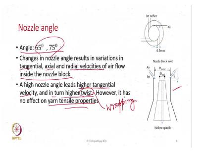
Now, nozzle angle, see here the diagram is shown here. The nozzle block inlet and this is the spindle, hollow spindle, and these are the nozzle, before nozzles and they are placed at an angle. This angle typically is 65 degree or 75 degree or may be some other value, but typically these are the angles.
