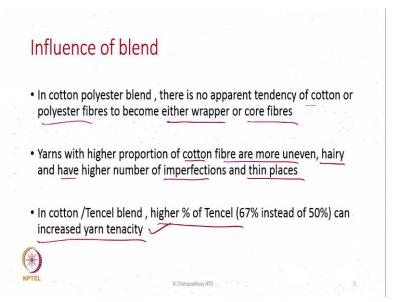
The another one we come to blend, in cotton polyester blend there is an no apparent tendency of the cotton or the polyester fibres to become either wrapper or core fibres. That means, if the sliver has cotton and polyester both, and they are intimately mixed, then each fibre has equal probability to make wrapper or becomes a part of core. See, probability of becoming a wrapper or becoming a core is same for both polyester and cotton fibre.
