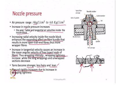
Now, we go to the one of the most important parameters that is nozzle pressure. So, if the pressure is increased the velocity of the air which is entering the nozzle is also going to increase. Typically, air pressure ranges between 4 kg force per centimeter square to 6 kg force per centimeter square.
