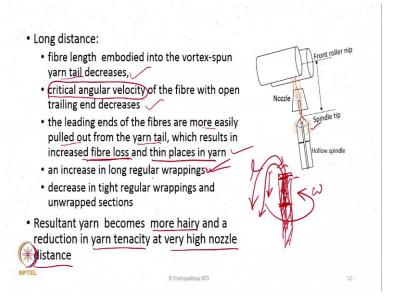
And if you go to the other extreme that is the longer distance, fibre length embodied in the vortex-spun yarn tail will decrease. Critical angular velocity of the fibre with open trailing end is going to also decrease. The leading ends of the fibres are more easily pulled out from the yarn tail, which results in increased in fibre loss and thin place in the yarn.
