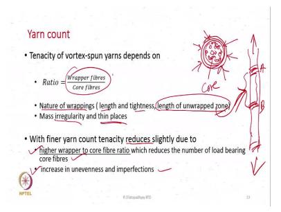
Now, we come to yarn count we can make a finer yarn, we can make a coarser yarn. The count range, I have already said it can vary between 15 to 65 Ne that is the range in which the yarns are spun.
