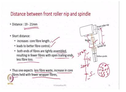
The other important parameter is the distance between the front roller nip and the spindle. It is shown in this diagram, so this is the distance. Front roller nip and the spindle tip is here. This distance is typically could be 19 to 21 millimeters. So, shorter the distance means it increases core fibre length, part of the fibre that is see the all the fibres are not forming wrappers.
