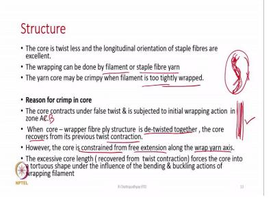
Now, the next topic is structure of such yarn and you can always automatically you can now visualize how the yarn will look like. In the core which will be almost 95, 96, 97 percent of the fibres will be forming the core and these fibre will be almost straight and parallel.
