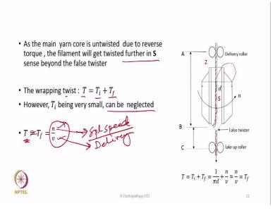
And they become straight and parallel and as the core is reverse twisted, the filament will get twisted further in the S directions; so, earlier there were little wrap in S directions. Now, they it will receive more wraps in the same S directions now; so, total wrapping twist therefore, will be T is going to  $T_i + T_f$ . However,  $T_i$  is very very small,  $T_i$  is only  $1/\pi d$  and therefore, it can be neglected for all practical purpose.
