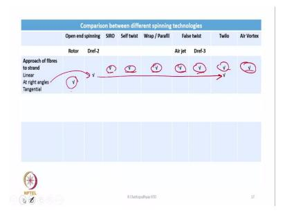
Approach of fibres to strand linear at right angles or tangential, so, these are basically linear, the next line is at right angles. So, right angles actually basically is this one that is Dref-2 and another right angle is there. This is end twilo that is there is a completely right 90 degree turn in the approach of fibres to the spinning or to the yarn formation position.
