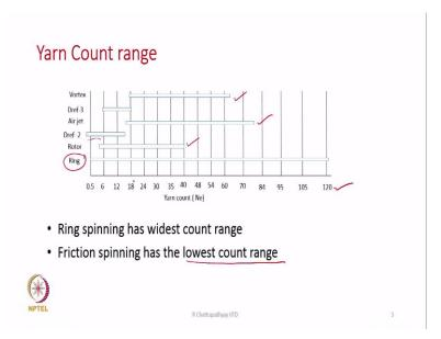
The yarn count range that can be produced, that is shown in this diagram. And, if you look at the most the bottom most which is the ring, you see there is a wide range starting from 0.5 Ne to 120 Ne. So, these bars are actually indicating the range of counts that can be produced. So, ring spinning has the widest count range.
