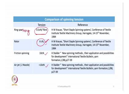
Here is a comparison of spinning tension. Spinning tension will be very high, in the case of ring spinning. So, I get a data where ring spun yarn or ring spinning process, the tension level was coated to be 0.3 cN/fibre. And, if there is a ring spun yarn we will be having at least 120 or 135 as depending upon the count, you can imagine even if we have 100 fibres, the spinning tension will go to 30 cN.
