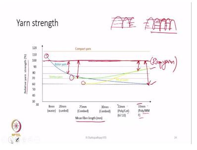
And here is a diagram which gives you the strength of the yarn. Yarn strength comparison as a function of mean fibre length. So, if we try to you know process this type of length of fibres 8 millimeter basically from waste material, 20 mm carded, 20 mm combed, 30 mm combed, 33 mm polyester cotton blend and 33 mm polyester manmade fibre blend. And if we produce yarns then we will find that the rotor yarn shown by this blue line.
