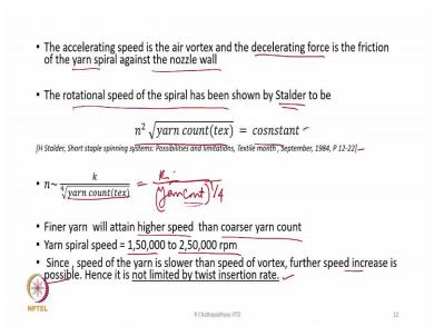
And the accelerating speed is the air vortex, but the decelerating force is the friction of the yarn spiral against the nozzle wall.
