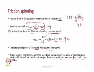
In friction spinning, friction drum is the source of the twist insertion to the yarn tail and speed of the yarn tail can be given by this equation, n Theoretical is D / small  $d_y$  into n D; D,  $d_y$  and n D these are given here.
