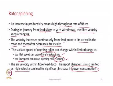
Now, rotor spinning is little interesting in this case. In rotor spinning an increase in productivity means, higher throughput rate. It is true for all spinning system, if we want to increase productivity means throughput rate is going to increase.
