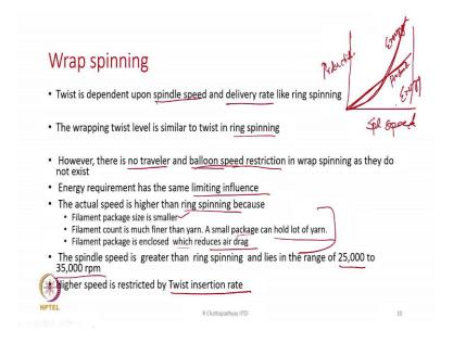
Next, we go to Wrap spinning; the wrap spinning is similar to ring spinning. So, twist is dependent on spindle speed and delivery rate like ring spinning. Wrapping twist level is similar to twist in ring spinning; however, there is no traveller in wrap spinning and there is no balloon. So, balloon speed restriction and traveller burning problems are not there in the case of wrap spinning, because they do not exist.
