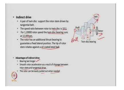
The other one is indirect drive as it is shown here a pair of twin disc support the rotor stem driven by a tangential belt. So, these two are the twin disc and here is the rotor and this is the rotor shaft, this is the rotor shaft. So, the rotor shaft is placed in between in the nip of the twin disc bearing and then the twin disc, disc 1 and disc 2, this is disc 1, this is disc 2, these two discs are actually in contact with a tangential belt and the belt is driven by a motor.
