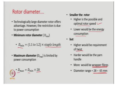
Technologically large diameter rotor offers advantages. However, the restriction is due to power consumptions, larger the diameter more is going to be the weight or the material remains same. So, though there are technological advantages we will discuss what are the advantages. Restriction is due to power consumptions.
