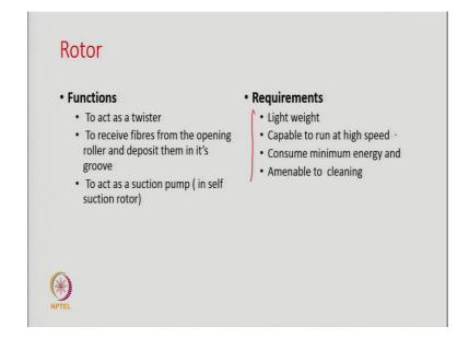
So, the rotor the main functions are to act as a twister, the second point is to receive the fibres from the opening roller and deposit them in its groove. So, it is acting as a collecting device and to act as a suction pump. Now, this is only in the case of self-suction rotor otherwise it is not does not act as a pump.
