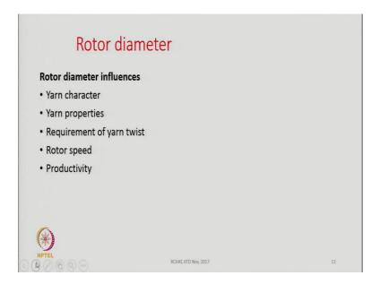
First we will discuss diameter, rotor diameter influences yarn character, it will also influence yarn properties, it can also have implication on the level of twist that we need to make sure that the spinning is going on smoothly or the spinning stability is there we are not encountering frequent breakages. It will also have effect on the rotor speed that we are going to choose and it can also have influence on the productivity.
