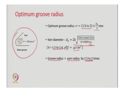
Now, groove what is the optimum radius of the grooves? If I look at the groove here as shown it here, this is the groove and these are the fibres, these are the fibres. So, optimum groove radius so, what should be the radius of this groove it has been stated to be 1.5 to 2 times the yarn radius,  $d_y/2$ , where ' $d_y$ ' is the diameter of the yarn.
