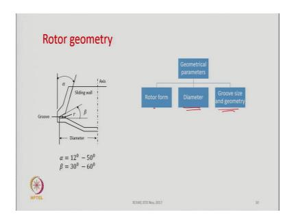
Now, rotor geometry, the rotor in a very simple term it is two cones attached at the base, but it is very important that what should be the inclination of the upper cone, what should the inclination of the bottom cone, these are important and we are going to discuss that. The geometrical parameters are form of the rotor, diameter and group size these three things are very very important.
