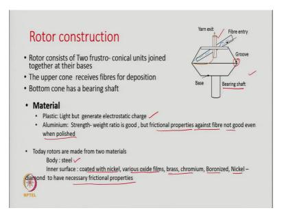
Now, rotor construction if we see in this diagram we are showing a typical simple sketch of the rotor. There is a base, there is a bearing shaft, then there is a fibre entry tube and there is another tube perpendicularly placed with respect to the rotor and through this the yarn is going to exit and here is the groove part.
