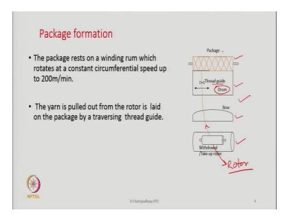
The package formation we are showing here a diagram which gives you an idea about how the package formation part looks like. So, here is the withdrawal or take up roller and then there is a bow we will come to that why this bow is required and then we have the winding drum there is a thread guide and the package rest on the winding drum.
