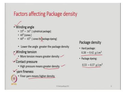
Now, factors affecting package density typically the winding angles are 33 to  $36^{\circ}$  for cylindrical package,  $40^{\circ}$  for cones and generally 40 to  $45^{\circ}$  for cones for package dyeing. Lower the angle greater is the package density, the winding tension more tension means greater density.
