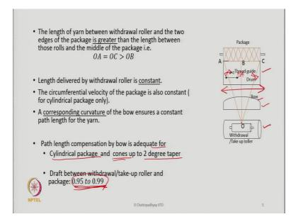
The thread guide which is there in between is doing a job what its continuously oscillating this thread guide is not is you know, which will be here in this position in the previous it is it could be here or it could be sometimes here or it could be sometimes here this is thread guide position. So, thread guides is actually guiding the yarn or laying the yarn on the surface of the package that is the job of the thread guide.
