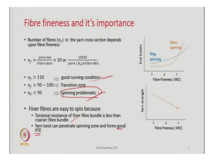
Today, we are now going to discuss Significance of Fibre and Process Parameters. We have already learnt about the rotor spinning machines, its working principles, and various parts or elements that makes this know particular machine. Now, we are going to discuss the importance of fibre parameters. So, first thing is you see the two diagrams are there on the right hand side. And the diagram shows fineness on one side and the other side end breaks fineness as well as yarn strength.
