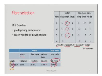
Fibre selection is based on spinning performance and quality needed for a given end use. Now, here a table where which is shown for different spinning system how the fibre parameters are important. So, for rotor spinning if we look at it for cotton, strength of the fibre is most important. That is rank one followed by rank two which is fineness of the fibre, the rank three is coming the length of the fibre.
