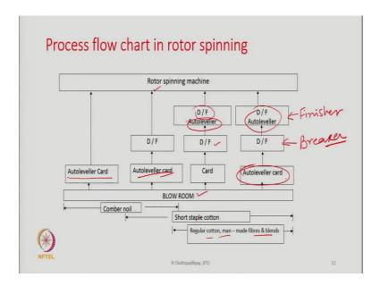
This gives a flowchart of the rotor spinning process you can say. So, the rotor spinning process flow chart is shown here that we start with short staple fibre or comber noil whatever we get or also we can take regular cotton man-made and fibres and blends. These are the 3 different types of machines also.
