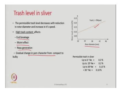
The other important fact is the trash level in this sliver, especially in the case of cotton. The permissible trash level decreases with reduction in rotor diameter and increases in its speed, and increase in its speed. That is if I go for higher speed my sliver should be very very clean.
