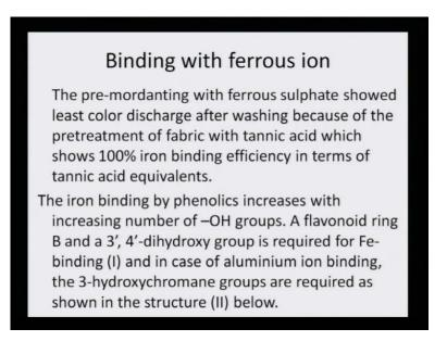
Binding with ferrous ion: The pre-mordanting with ferrous sulphate showed least color discharge after washing because of the pretreatment of the fabric with tannic acid which shows 100 percent iron binding efficiency in terms of tannic acid equivalents. The iron binding by phenolic increases with increasing number of OH. A flavonoid ring B and a 3
