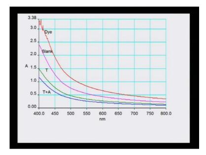
So, the optical density shows that the dye which was initially 3.38 as now reduced in the case, because all the dye has got transferred to the fabric. So, this is the kind of contribution the tannic acid make an mordants make.
