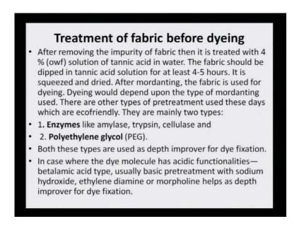
Treatment of fabric before dyeing: After removing the impurities of fabric then it is treated with 4 percent weight of the fabric solution of tannic acid in water. The fabric should be dipped in tannic acid this is for cotton dyeing when we are preparing for free treatment for cotton. Tannic acid is only and only used when cotton dyeing is carried out.
