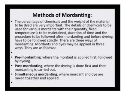
Methods of mordanting: Now, mordant ideally is should be used with the dye that we have understood, but whether to use it before dyeing as a pretreatment or whether it should be used together with the dyeing that is simultaneously or whether the mordanting should be done after dyeing that is post-mordanting or various other options that can be considered when one is trying to play around with different shades of dyeing.
