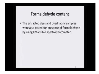
Formaldehyde analysis - The extracted dye, and dyed fabric samples were also tested for presence of formaldehyde by using UV visible spectrophotometer. Now, formaldehyde does not come from any you know source, but it is a part of that textile processing, where
