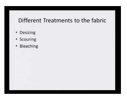
So, let us try to look at the procedure. Different treatments to the cotton fabric are it needs to be desized; it needs to be covered and it needs to be bleached finally. So, there are three main steps that cotton needs to undergo - one is desizing; the other one is scouring; and the third one is bleaching.
