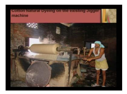
Now, this is a typical jigger machine where we used our natural dyeing process and you will see that a man is manually rotating the fabric, and the fabric is going in to the dye bath and at the same time the entire process is done in a such a fast manner that for a particular time not too long the fabric is in the dye bath. So therefore, and because it is in circulation the dye...
