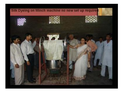
Similarly, this is a winch machine which was shown for silk dyeing. As I told you in the winch machine there are two wheels and cloth is actually rapped or like a rope and then put in to the dye bath there is a dye bath at the bottom, and it was showing very good dyeing results for silk and wool yard.
