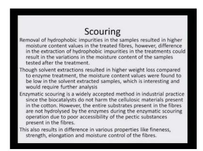
Scouring; therefore, removal of hydrophobic impurities in the sample resulted in higher moisture content values in the treated fibers; however, difference in the extraction of the hydrophobic impurities in the treatments could result in variations in the moisture content of the samples tested after the treatment. Though solvent extractions resulted in higher weight loss compared to enzyme treatment, the moisture content values were found to be low in the solvent extracted samples.
