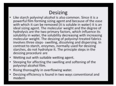
Like starch polyvinyl alcohol is also one of the common compounds. Since it is a powerful film coating sizing agent, and because of the ease with which it can be removed, it is soluble in water, it is an ideal sizing agent. So, apart from starch, there is an another compound called polyvinyl alcohol, which is also used as sizing agent; and therefore, it has to be removed too, and it the removal of polyvinyl alcohol is much easier, because it is water soluble.
