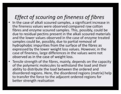
Effect of scouring on the fineness of the fabric: In case of alkali scoured samples, a significant increase in the fineness values were observed; compared raw cotton fibers and enzyme scoured fibers, this possibly could be due to residual pectin's present in the alkali scoured materials, and the lower values observed in the case of enzyme treated samples could be possibly due to partial removal of hydrophobic impurities from the surface of the fiber as expressed by the lower weight loss values.
