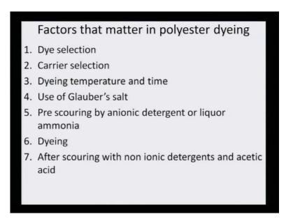
Factors that matter the polyester dyeing is dye selection, carrier selection, if we are not following the thermosol process, dyeing temperature and time, use of Glauber's salt for
