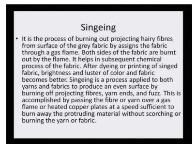
Singeing: It is a process of burning out projecting hairy fibers from surface of the grey fabric, by assigns that fabric through a glass flame; both sides of the fabric are burnt out by the flame; it helps in subsequent chemical process of the fabric, after dyeing or printing of singed fabric brightness and luster of the color, and fabric becomes better. Singeing is a process applied to both yarns and fabrics to produce an even surface by burning off projecting fibers, yarn ends and fuzz.
