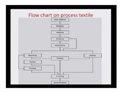
A grey material; this the usual flow chart; a gray material goes through singeing, desizing, scouring, merserizing. And then it goes through bleaching, dyeing, printing or it can go to dyeing or it can go to printing and finally to finishing, and to the finish good. So, this the flow charts, so there are several, several steps, which need to be understood clearly as to what is their role.
