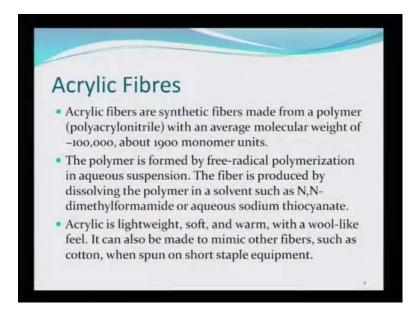
Acrylic fibers: Acrylic fibers are synthetic fibers made from a polymer; that is polyacrylonitrile with an average molecular weight of 100000 about 1900 monomer units being linked up. So, you see it is a macromolecule first thing made out of polyacrylonitrile;
