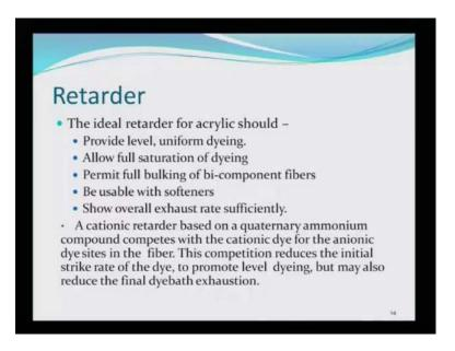
So, these retarders the ideal retarder for acrylics are it should provide level uniform dyeing, allow full saturation of dyeing, permit full bulking of bi-component fibers, be usable with softeners, show overall exhaust rate sufficiently. Because the rate of adsorption, and the rate of penetration should be even. If the rate of adsorption is fast, the dye will aggregate and that much has not penetrated. So, it will cause uneven un that many sites are not available for electrostatic attraction.
