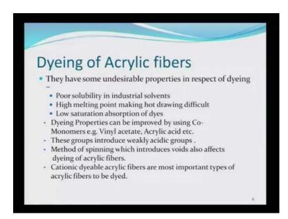
Dyeing of acrylic fiber: They have some these undesirable properties in respect of dyeing, and those need to be taken in into account what is the problem? That needs to be addressed while dyeing an acrylic fiber. They have poor solubility in industrial solvents, high melting point making hot drawing difficult, low saturation absorption of dyes; dyeing properties can be improved by using co-monomers like vinyl acetate acrylic acid.
