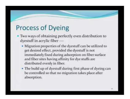
The process of dyeing: Two ways of obtaining perfectly even distribution to dyes of dyestuff in acrylic fiber. Now, you see that there are possibilities the dye aggregates may form. So, how can one attain a very perfect method of dyeing. Migration properties of the dyestuff can be utilized to get desired effect provided the dyestuff is not immediately fixed during adsorption on surface, fiber surface and the fiber sites having affinity for dye stuffs are distributed evenly in the fiber.
