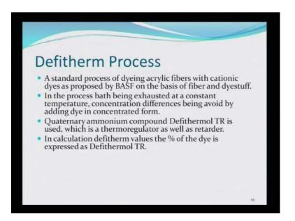
So, that is why there is a the process must be standardized, and a process standardized by BASF called the Defitherm process for dyeing of acrylic fiber has also been established.
