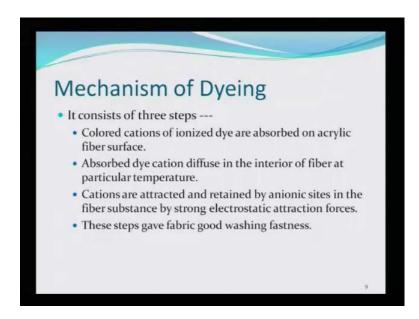
Mechanism of dyeing: It consists of three major steps; colored cayions of ionized dye are absorbed on acrylic fiber surface, absorbed dye cation diffuse in the interior of fiber at particular temperature.
