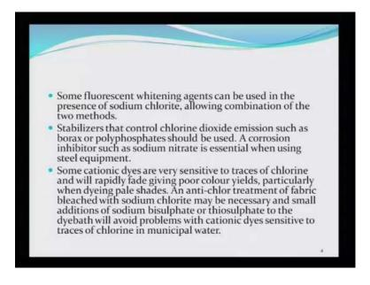
Some fluorescent whitening agents can be used in the presence of sodium chlorite, allowing combination of the two methods. So, it is possible to use fluorescent, whitening agent and bleaching agent together, but may be not an all types of combination. So, one has to carefully choose the different re-agents as what I mentioned a while ago, the anionic and the cationic detergents cannot be used. So, a non ionic detergent is used for washing.
