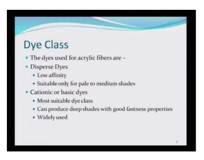
The type of dyes that can be used with acrylic acid or acrylic fiber is very important to be understood. Not every dye can be used, now you understand, because this has to have cationic nature dye, because the fiber is more anionic in nature.
