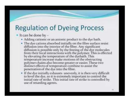
Regulation of dyeing process: It can be done adding cationic or an anionic product to the dye bath the dye cations absorbed, initially on the fiber surface resist, the diffusion into interior of the fiber. Any significant diffusion is possible only by the freeing the dye molecules from the local interactions with the polymer. This is effected by elevating the temperature of the dye bath, this in temperature increase makes motions of the obstructing polymer chain also become greater or easier.
