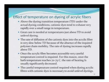
The effect of temperature we have already seen that above the dyeing transition temperature under the actual dyeing condition, cationic dyes tend to exhaust very rapidly. Great care is needed at temperature just above the transition temperature to avoid unlevel dyeing. The rate of diffusion of cationic dyes into the acrylic fiber is very slow below the transition temperature, because of the absence of the required polymer chain mobility.
